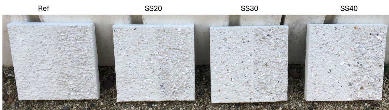
Figure 1. Surface appearance of concrete slabs after sandblasting (2 different sandblasting levels for the same sample).
