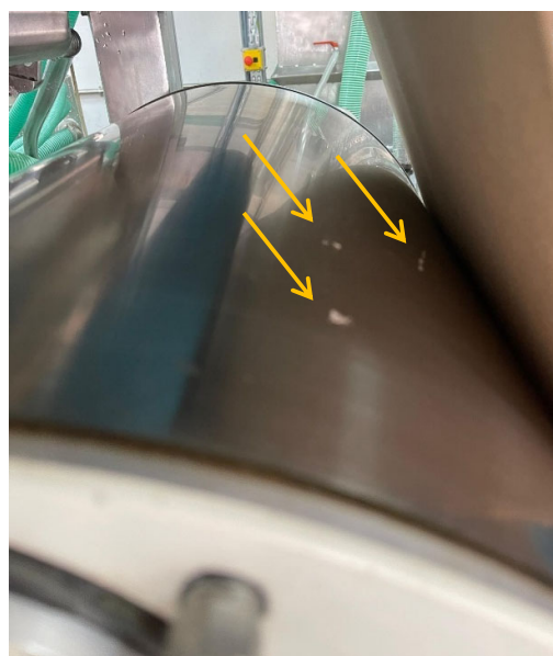
Figure 1. Photograph showing the adhesion of the sheet to the first drying cylinder at the machine's highest speed (5 m/min).
