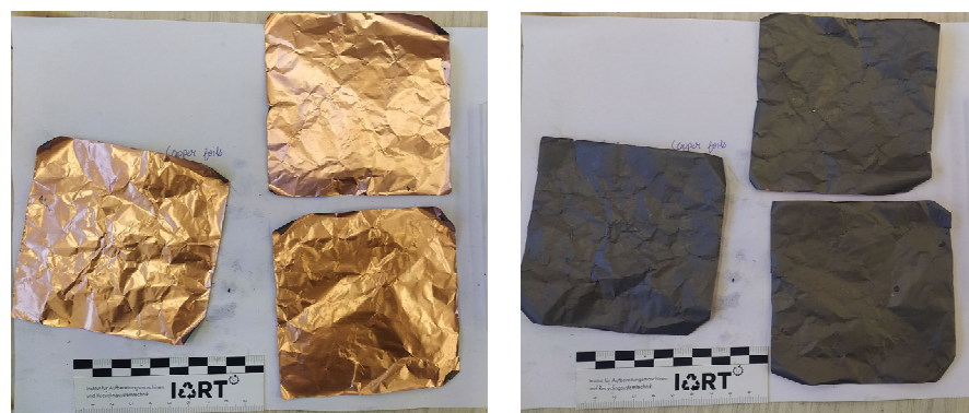
Figure 4. The 10 × 10 cm particles after delamination at 80 °C: the front side ( left ) shows the smooth, delaminated surface, while the back side with the rough surface ( right ) remains coated.
