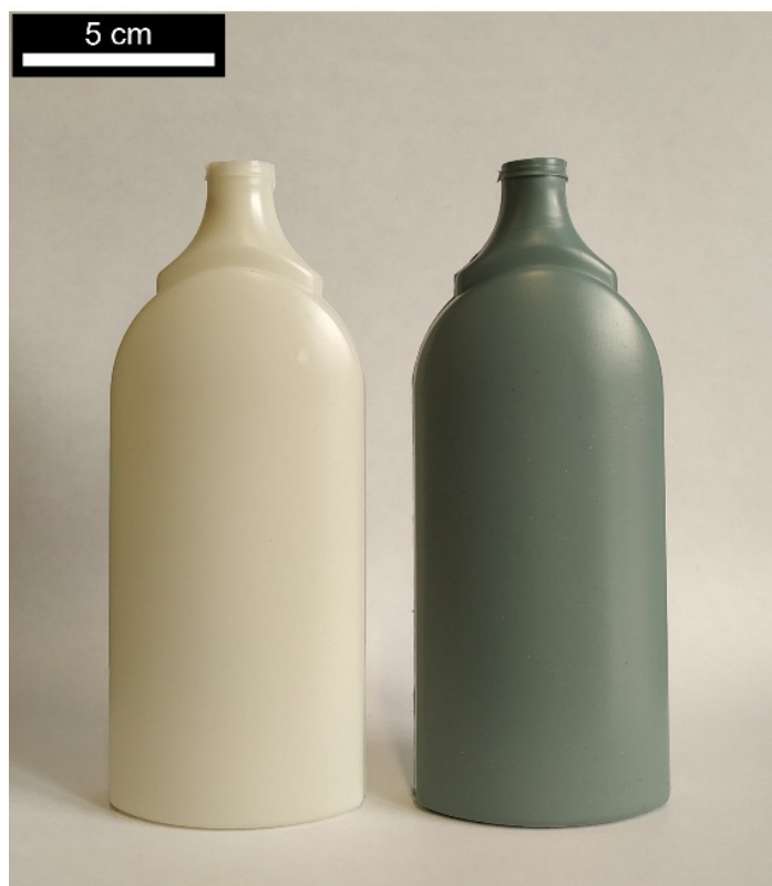
Figure 12. Extrusion blow-moulded rPE–HD bottle prototypes (100% regranelate).
