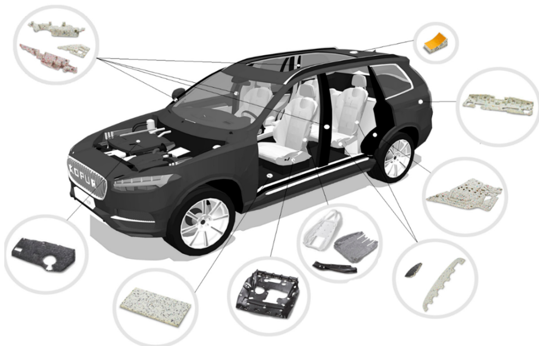
Figure 3. Acoustic filler in vehicle interiors and filler for car seats.
