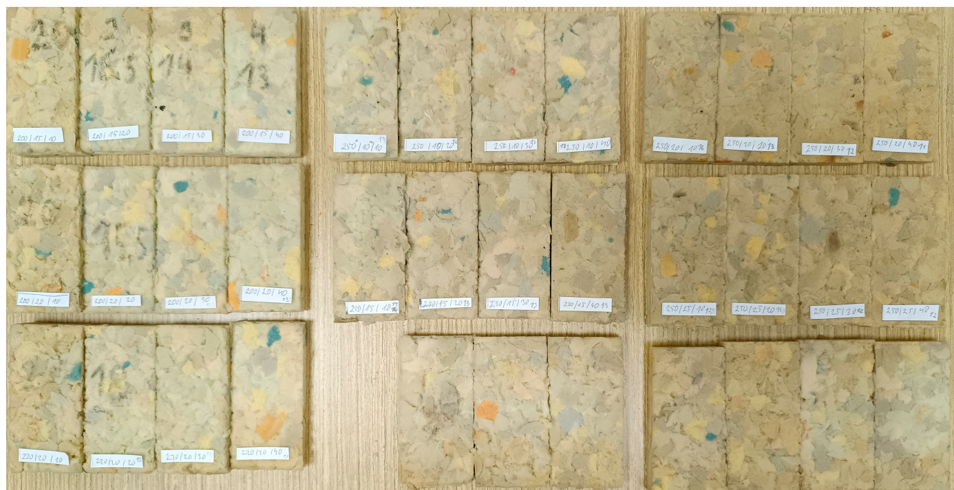
Figure 10. Test samples in the dry compression moulding experiment. Sample marking: Heating temperature (°C)/Heating period (min)/Pressing pressure (kPa).
