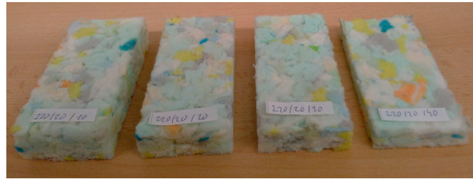
Figure 9. Removal of finished samples from the mould. Different loads represent different heights.
