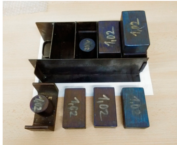
Figure 6. Mould and weights for the production of experimental samples.
