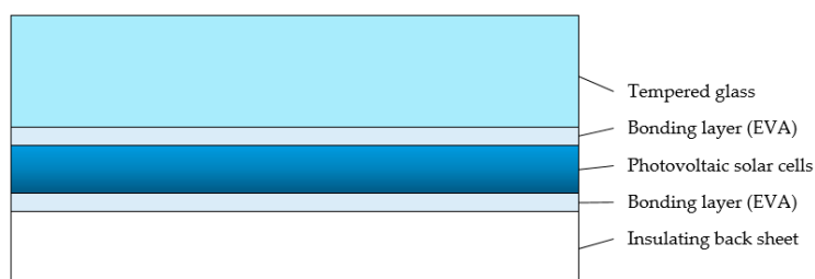
Figure 8. (a) Test sample from an obsolete single-sided PV panel; (b) scheme of the cross-sectional structure of the panel used for the tests.
