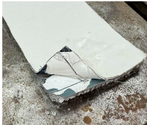
Figure 2. Partially separated insulating back sheet.
