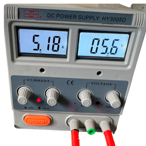
Figure 9. (a) Manual proof-of-concept test device with a metal wire; (b) DC Power Supply HY3005D during testing.
