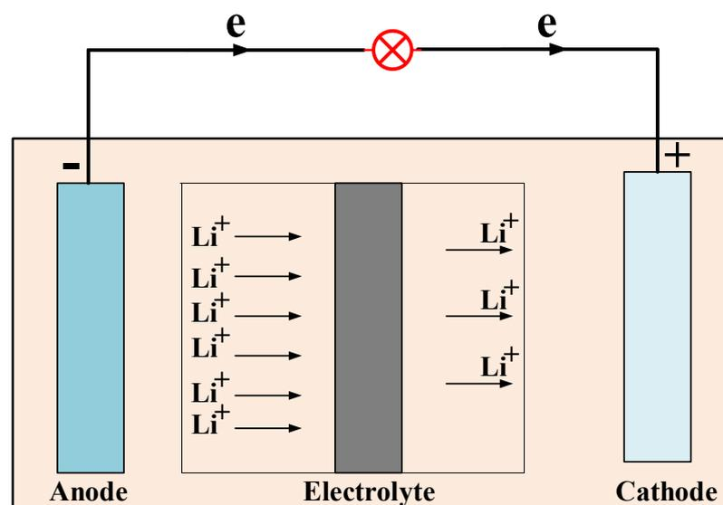
Figure 2. Components of a rechargeable Li-ion battery [58].
