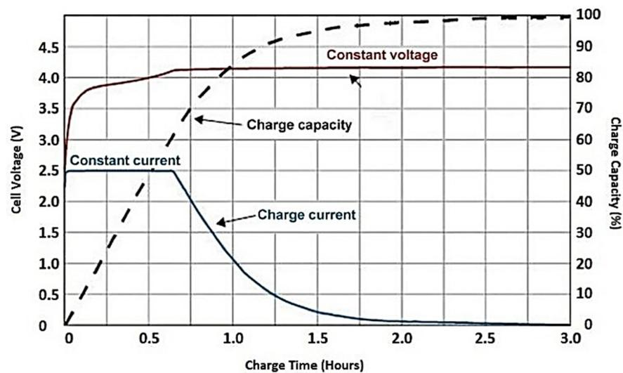
Figure 3. Volts/capacity vs. time during the charging of lithium-ion [70].
