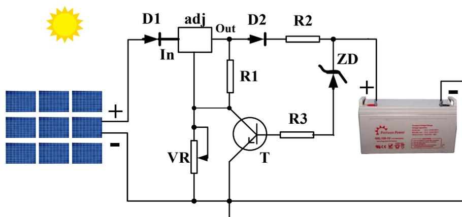
**Figure 1.** A schematic diagram of the solar battery charging circuit.
