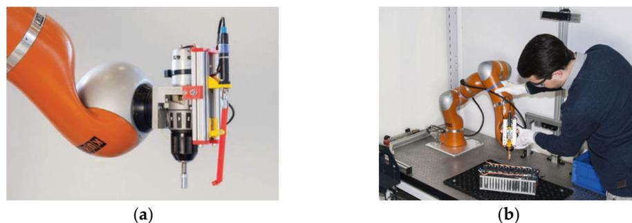
**Figure 14.** Semi-automated disassembly: (a) Prototype of screwdriving tool without housing, and (b) implementation of the hybrid disassembly workstation. Copyrights: (a) Figure captured from [87] without any change, reprinted with permission from Elsevier; (b) Figure captured from [88] without any change, reprinted with permission from Reinhart, Handbuch Industrie 4.0, © 2017 Carl Hanser Verlag GmbH & Co. KG., Munich, Germany.
