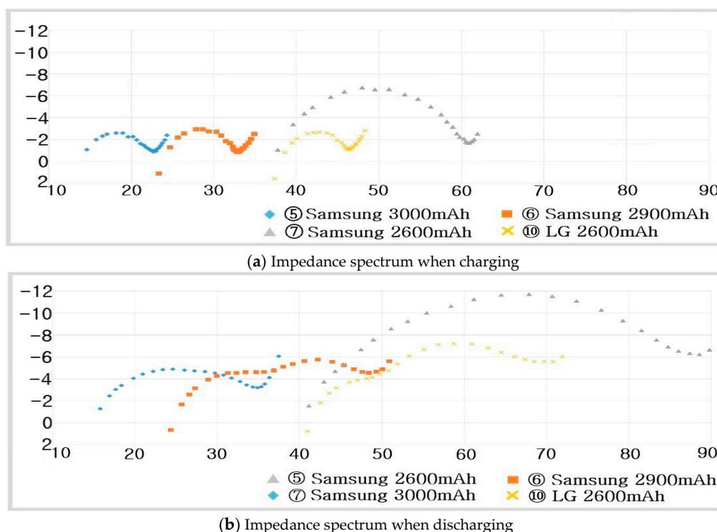
Figure 18. Impedance spectra of 18650-type Li-ion batteries (non-protection device).
