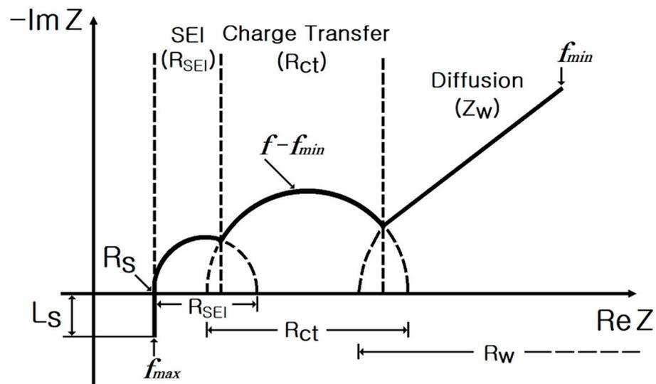
Figure 4. Complex plane diagram of the impedance spectrum of a cylindrical Li-ion battery [5,7].
