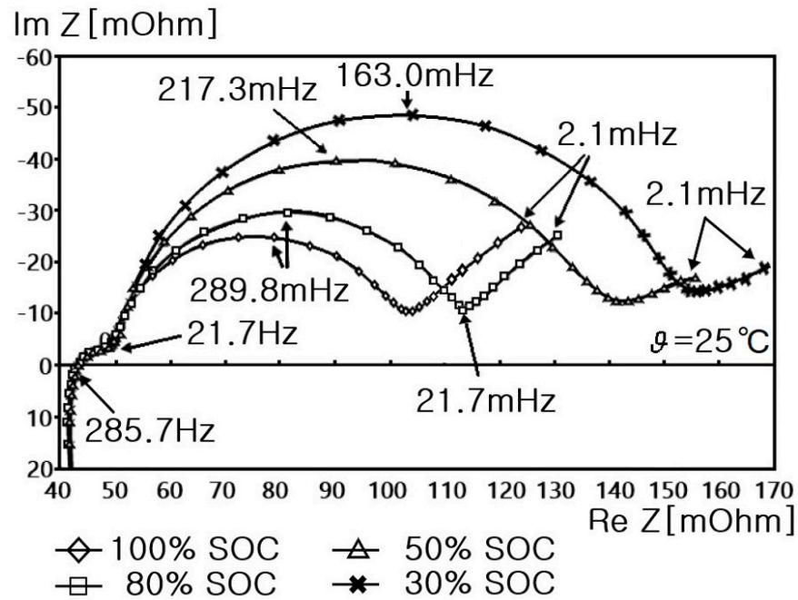
Figure 6. Impedance spectrum according to the SoC of a cylindrical Li-ion battery [5].
