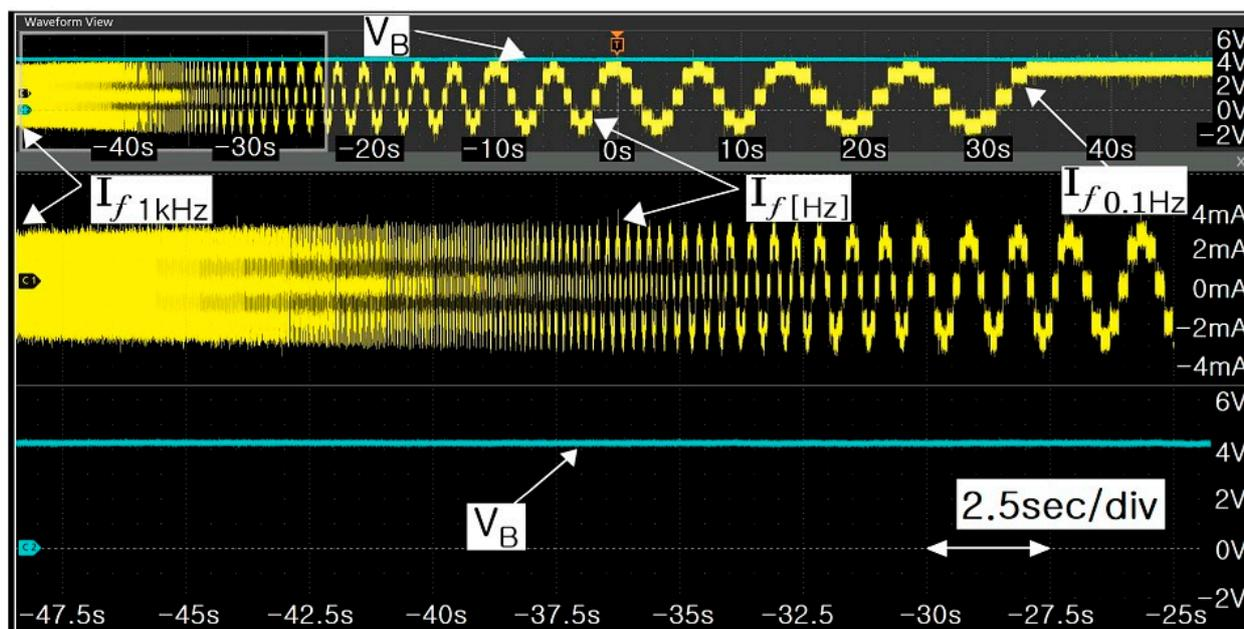
Figure 16. Voltage and current waveforms when measuring impedance spectrum.
