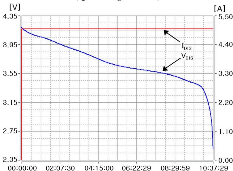
(b) Discharge voltage and current waveforms for a pouch-type Li-ion battery (Ⓐ Shenzhen Aoyouji Energy 50.5 Ah)
