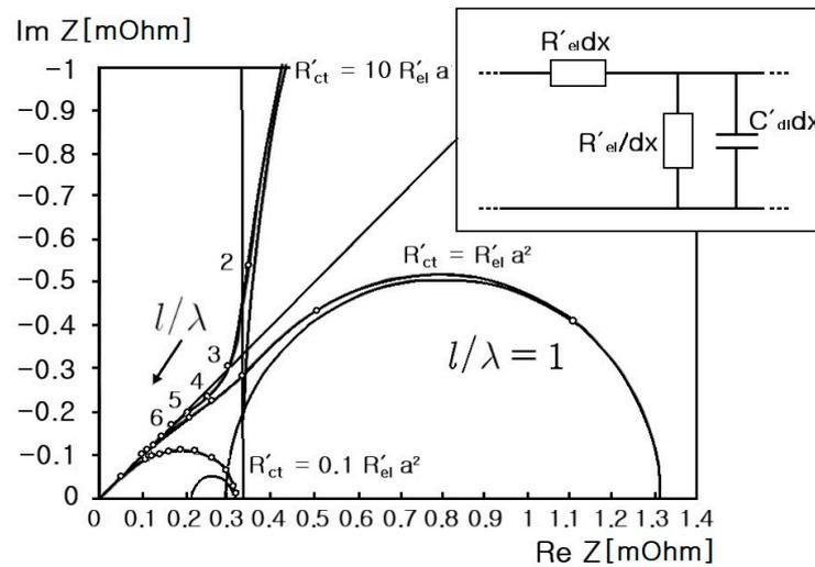
**Figure 13.** Theoretical model of the impedance spectrum of supercapacitors with porous electrodes [11].
