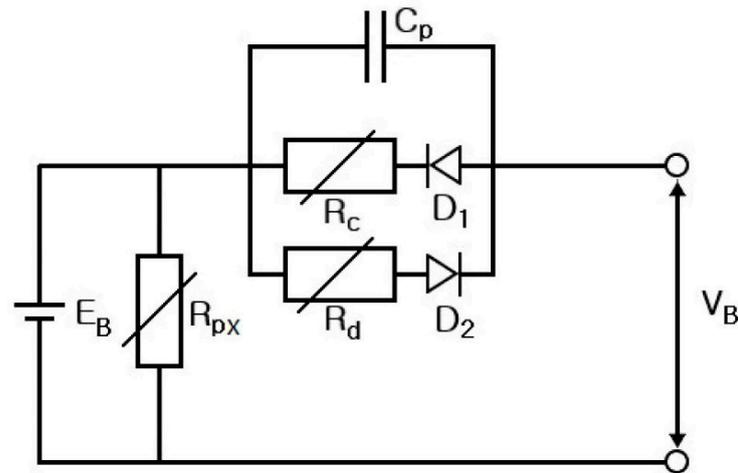
Figure 3. Improved battery model [3,4].
