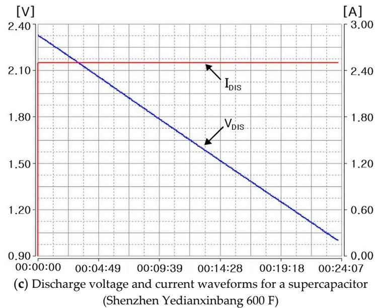
**Figure 25.** Discharge voltage and current waveforms of Li-ion batteries and supercapacitor.
