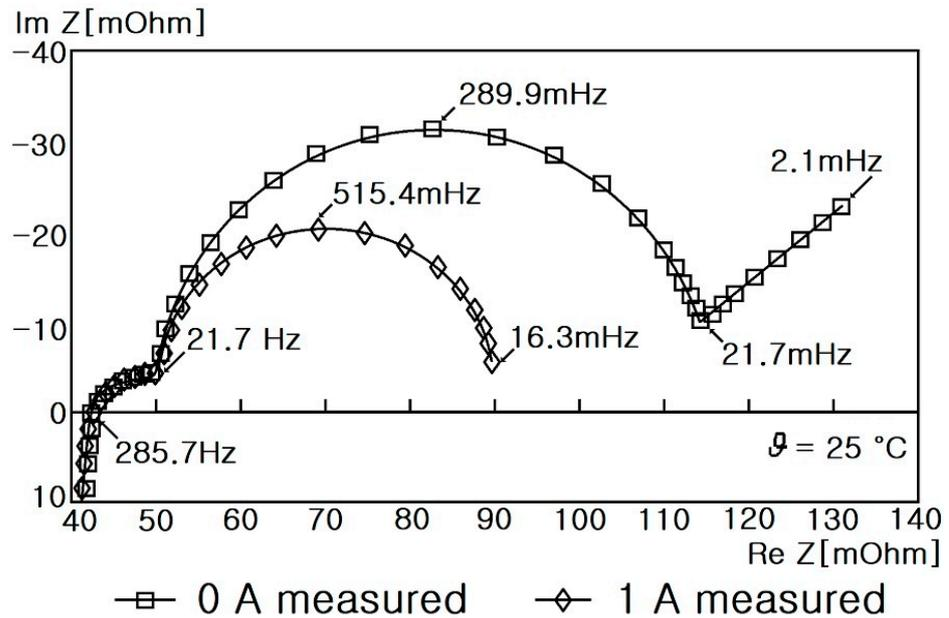
Figure 7. Impedance spectrum according to the presence or absence of charging for a cylindrical Li-ion battery [5].
