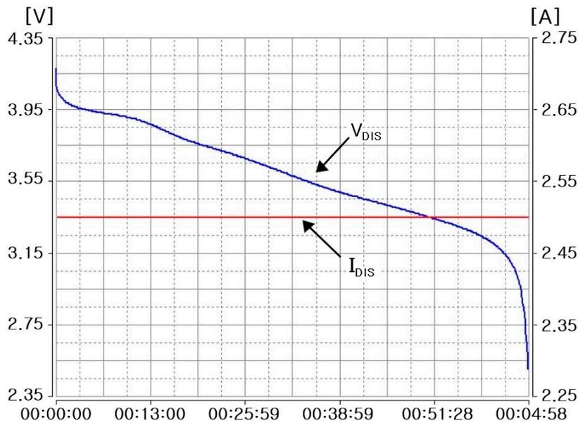
(a) Discharge voltage and current waveforms for a cylindrical Li-ion battery (Ⓞ Samsung 2900 mAh)
