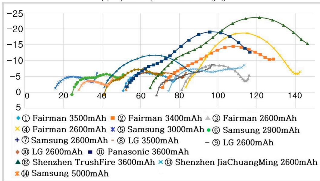
(b) Impedance spectrum when discharging
