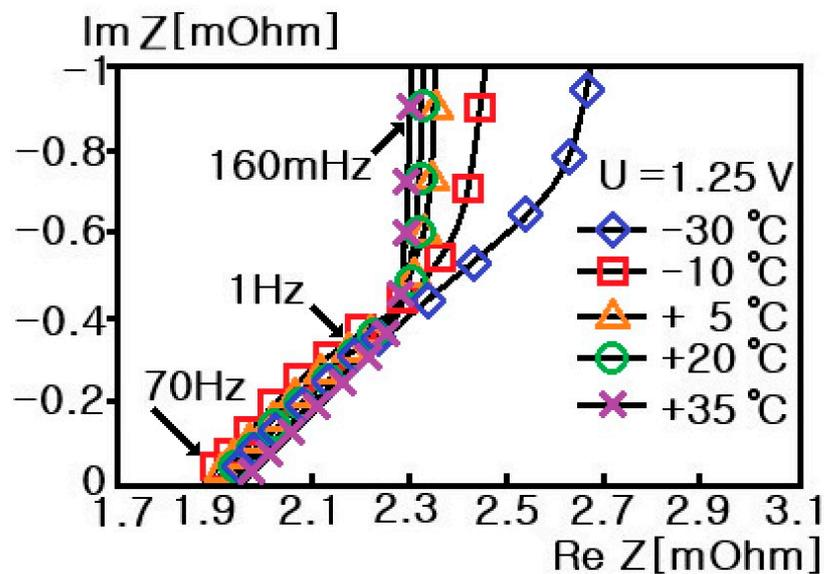
Figure 9. Impedance spectrum according to temperature of the supercapacitor [5,6].
