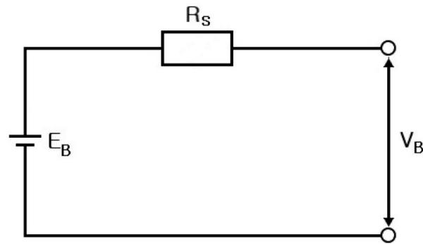
Figure 1. Simple battery model [1].
