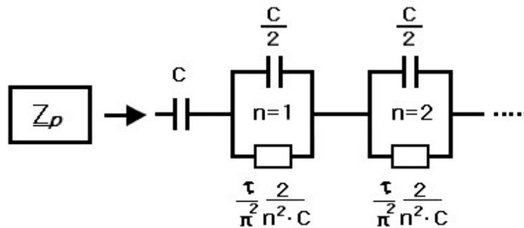
Figure 11. Electrical equivalent model of the supercapacitor impedance ( $Z_{-p}$ ) [6].
