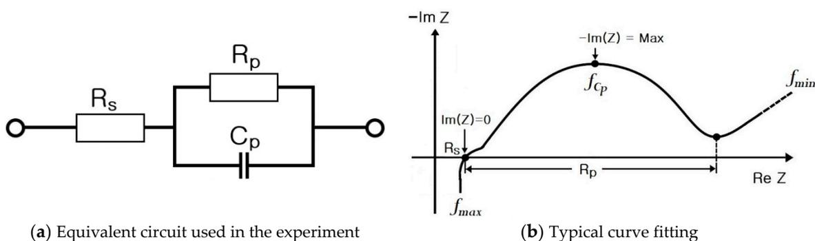
Figure 17. Equivalent circuit and typical curve fitting.
