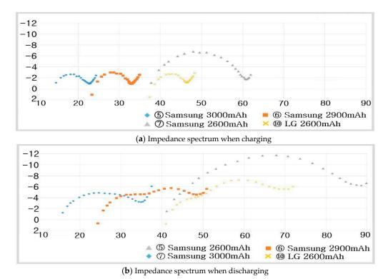
Figure 18. Impedance spectra of 18650-type Li-ion batteries (non-protection device).
