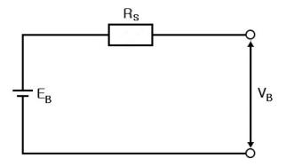
**Figure 1.** Simple battery model [1].
