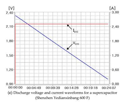
Figure 25. Discharge voltage and current waveforms of Li-ion batteries and supercapacitor.
