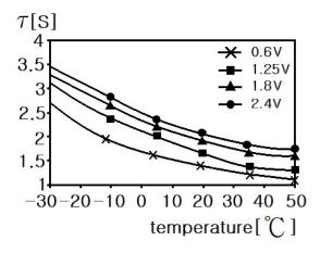
**Figure 12.** Curve of  $\tau$ , which is an independent parameter of temperature and voltage in supercapacitors.
