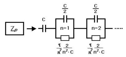
**Figure 11.** Electrical equivalent model of the supercapacitor impedance  $(Z_p)$  [6].
