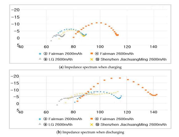
Figure 20. Impedance spectra of 2600 mAh 18650-type Li-ion batteries (built-in protection device).
