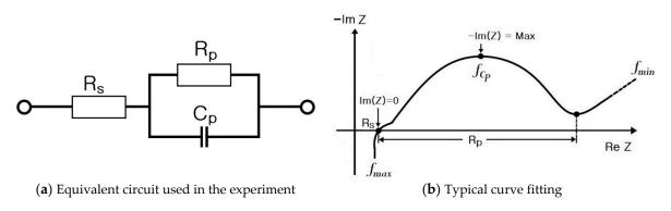
Figure 17. Equivalent circuit and typical curve fitting.
