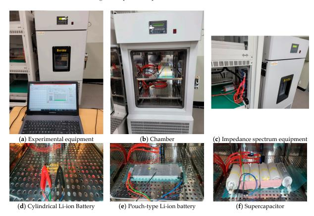
Figure 15. Experimental apparatus.
