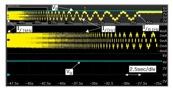
Figure 16. Voltage and current waveforms when measuring impedance spectrum.
