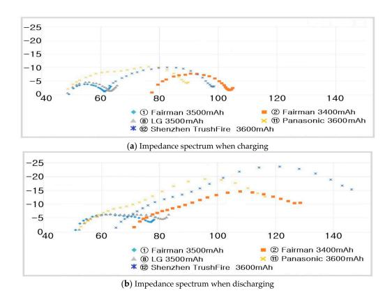
**Figure 19.** Impedance spectra of 18650-type (cylindrical 3400–3600 mAh) Li-ion batteries (built-in protection device).
