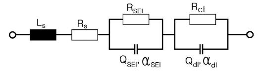
**Figure 8.** Electrical equivalent circuit of pouch-type Li-ion battery.
