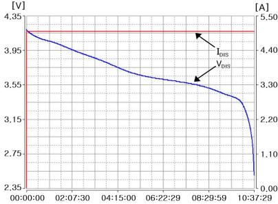
(b) Discharge voltage and current waveforms for a pouch-type Li-ion battery (A) Shenzhen Aoyouji Energy 50.5 Ah)
