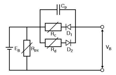
Figure 3. Improved battery model [3,4].
