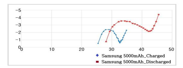
Figure 21. Impedance spectrum of 21700-type Li-ion Batteries (built-in protection device).
