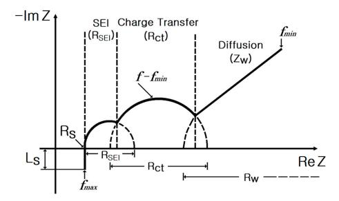
**Figure 4.** Complex plane diagram of the impedance spectrum of a cylindrical Li-ion battery [5,7].
