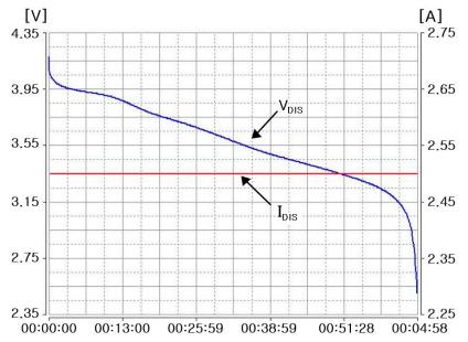
(a) Discharge voltage and current waveforms for a cylindrical Li-ion battery (6) Samsung 2900 mAh)
