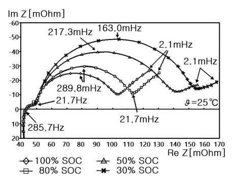
Figure 6. Impedance spectrum according to the SoC of a cylindrical Li-ion battery [5].
