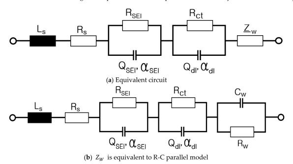
Figure 5. Electrical equivalent circuit of a cylindrical Li-ion battery.
