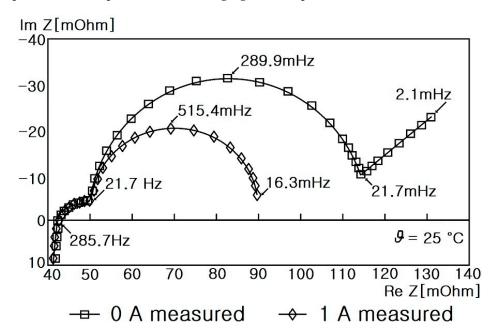
**Figure 7.** Impedance spectrum according to the presence or absence of charging for a cylindrical Li-ion battery [5].
