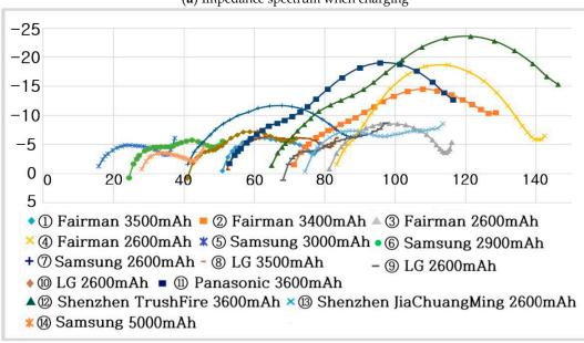
(b) Impedance spectrum when discharging
