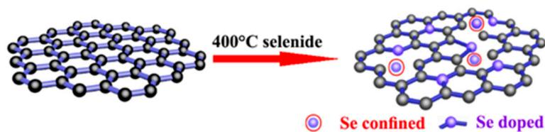
**Figure 1.** Synthesis principal of Se@SCDC composites.
