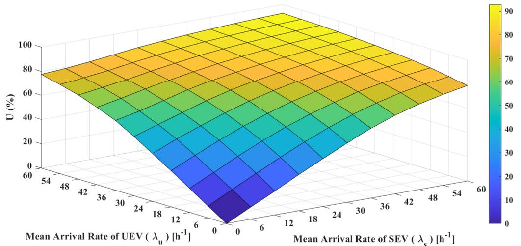
Figure 5. Charging resource utilization with  $\lambda_s$  and  $\lambda_u$ .
