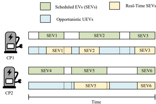
**Figure 2.** Utilization of charging resources by UEVs.
