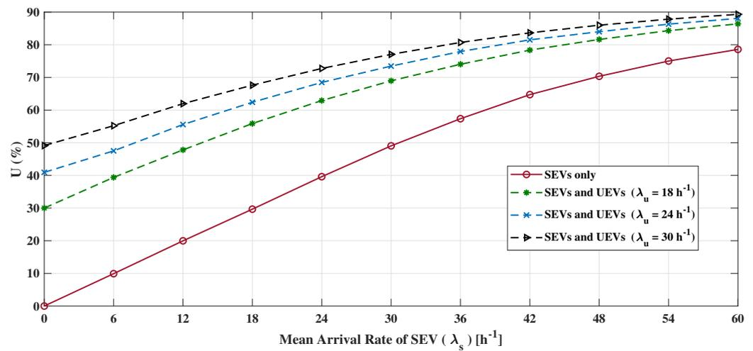
Figure 4. Charging resource utilization with  $\lambda_s$ .
