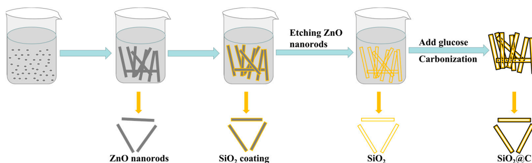
Scheme 1. Synthesis illustration of the nanotubular \text{SiO}_2@\text{C} composites.
