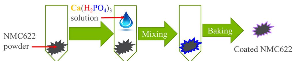
**Figure 1.** Schematics of wet impregnation for depositing functional surface coating on NMC622 (LiNi<sub>0.6</sub>Mn<sub>0.2</sub>Ni<sub>0.2</sub>O<sub>2</sub>).
