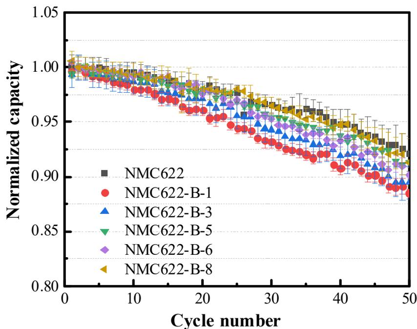
**Figure 6.** Discharge capacity of half cells during charge/discharge cycling between 2.5 V and 4.4 V with a constant current of C/3 for  $\text{LiNi}_{0.6}\text{Mn}_{0.2}\text{Co}_{0.2}\text{O}_2$  with and without modification with  $\text{H}_3\text{BO}_3$ . The concentration of  $\text{H}_3\text{BO}_3$  in the solution is 1 wt% (NMC622-B-1), 3 wt% (NMC622-B-3), 5 wt% (NMC622-B-5), 6 wt% (NMC622-B-6), and 8 wt% (NMC622-B-8), respectively.
