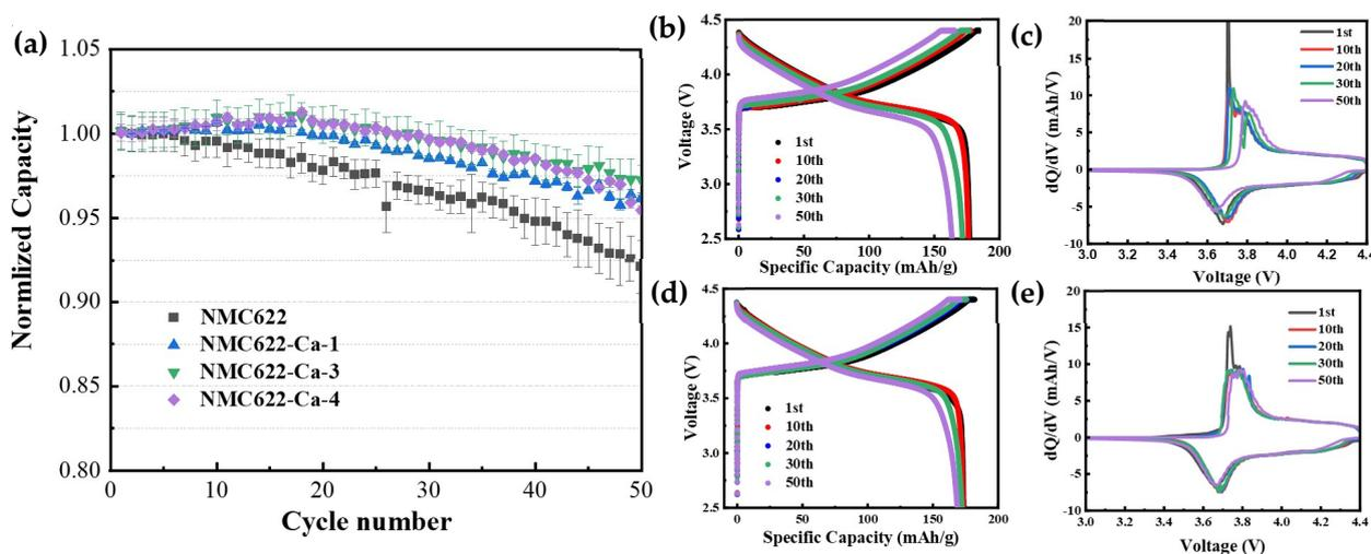
**Figure 4.** (a) Discharge capacity of half cells during charge/discharge cycling between 2.5 V and 4.4 V with a constant current of  $C/3$  ( $\sim 1$  mA), showing the impact of  $\text{Li}_3\text{PO}_4/\text{Ca}_3(\text{PO}_4)_2$  coating on the performance of NMC622. (b) Voltage profile of NMC622 and (c) corresponding  $dQ/dV$ . (d) Voltage profile of NMC622-Ca-3 and (e) corresponding  $dQ/dV$ . Please note the 1st cycle is taken after formation cycles.
