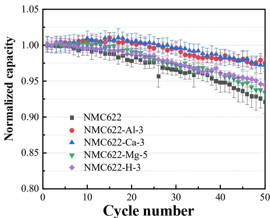
**Figure 5.** Comparison of the capacity retention of NMC622 processed with different acidic phosphate-based solutions.
