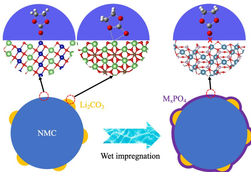
**Figure 7.** Schematics illustrates the mechanism for stabilized cathode/electrolyte interface with the functional surface coating.
