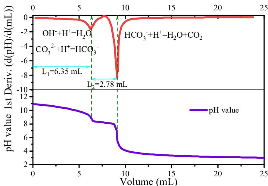
**Figure 2.** Titration curve to determine the level residual  $\text{LiOH}/\text{Li}_2\text{CO}_3$  in  $\text{LiNi}_{0.6}\text{Mn}_{0.2}\text{Co}_{0.2}\text{O}_2$ .
