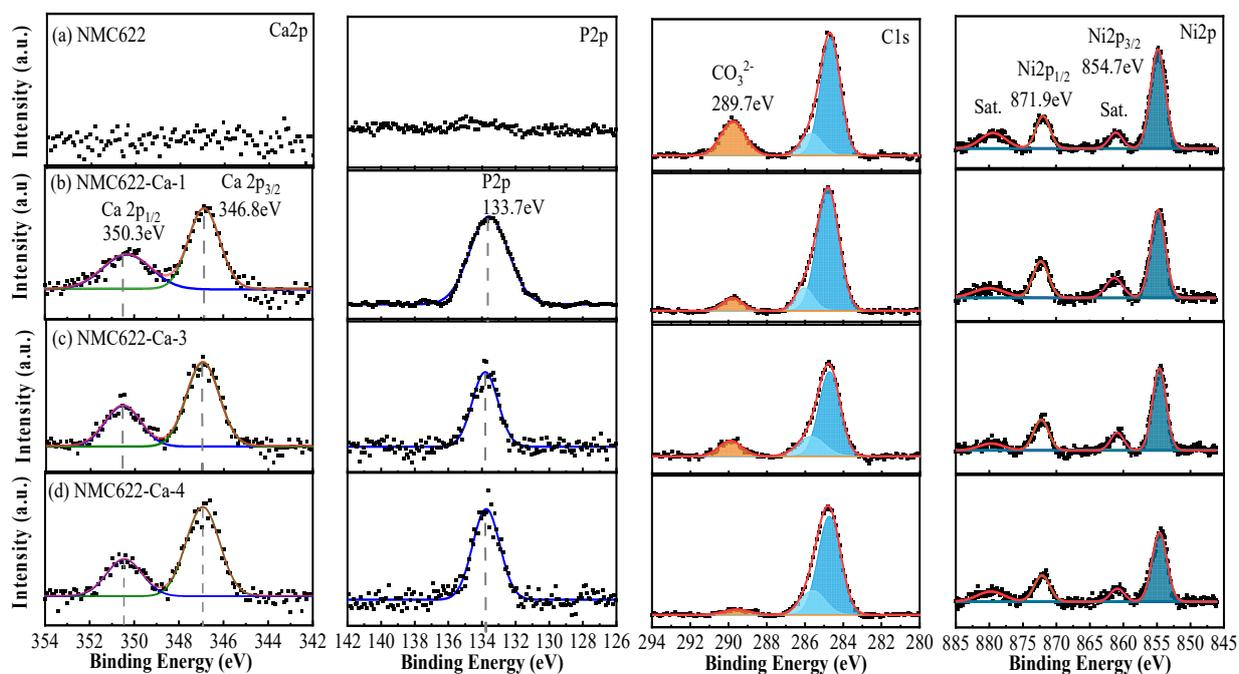
**Figure 3.** XPS results showing the deposition of phosphates on the surface of (a) pristine NMC622; (b) NMC622-Ca-1; (c) NMC622Ca-3; and (d) NMC622-Ca-4. Dotted lines represent raw spectrum and solid lines represent fitted spectrum. Some peak areas were colored to guide reader.
