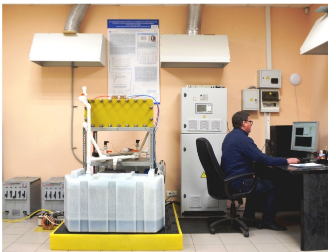
Figure 2. 6 kWh VRB test bench.
