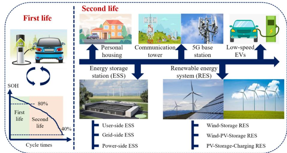
Figure 12. Typical echelon utilization scenarios of retired power LIBs.
