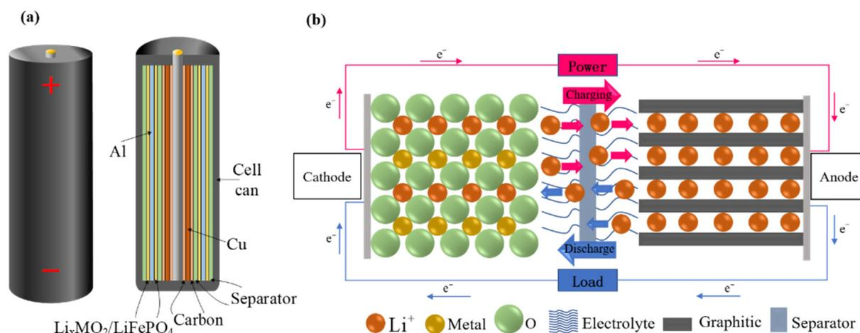
**Figure 3.** A schematic diagram of a cylindrical LIB's shape, composition, and charging and discharging process (a) Shape and composition of cylindrical LIB. (b) Schematic diagram of the charging and discharging process of LIB.
