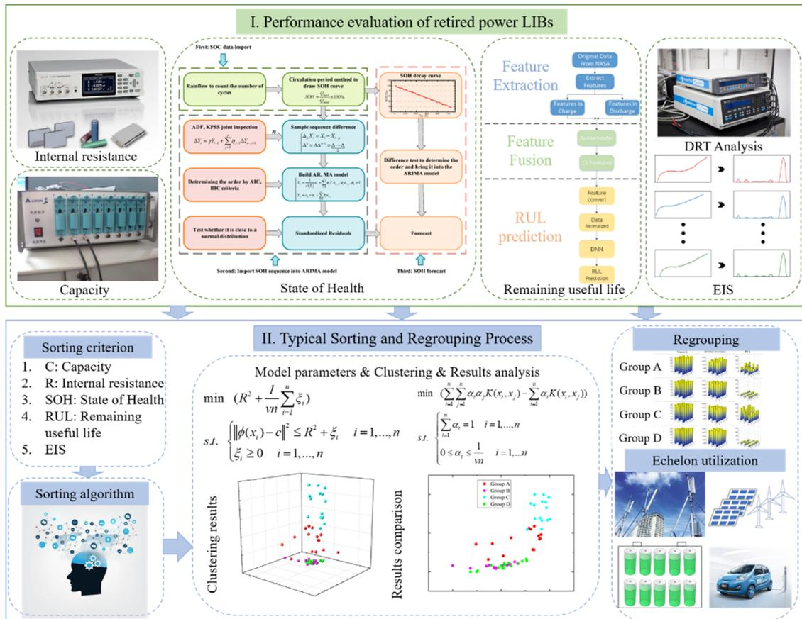
Figure 11. A typical sorting and regrouping framework for retired power LIBs [89].
