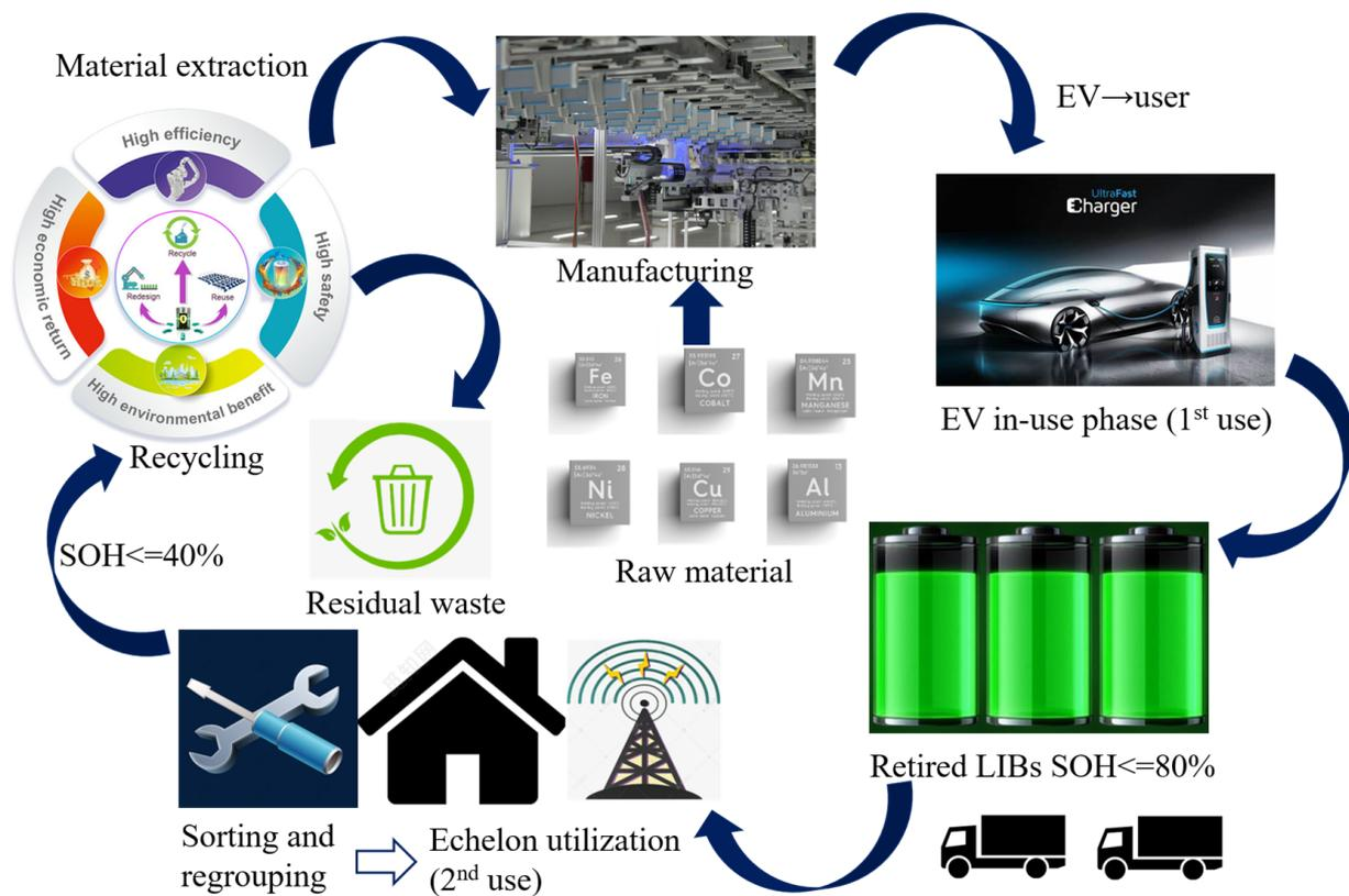
Figure 5. Disposal route for echelon utilization of retired power LIBs.
