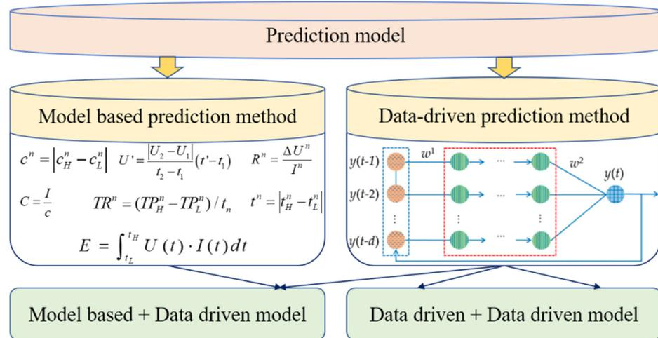
Figure 10. Framework for the hybrid-driven approach of RUL prediction [65].
