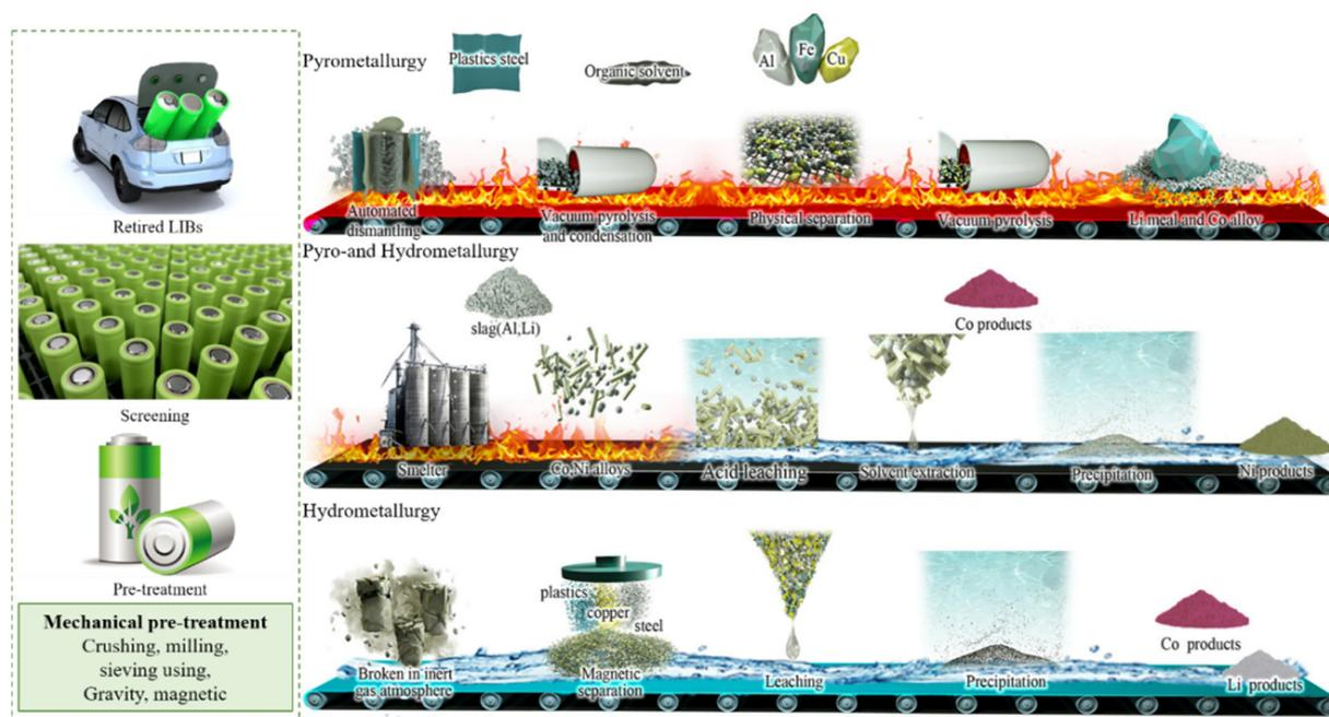
**Figure 4.** Process flow of industrial recycling method (pyrometallurgical, hydrometallurgical and pro-and hydrometallurgical) of retired power lithium battery (Ref. [1]).
