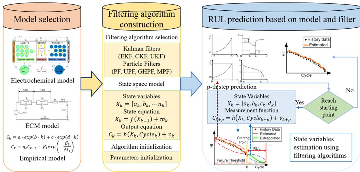
Figure 8. Framework for the model-based approach of RUL prediction.
