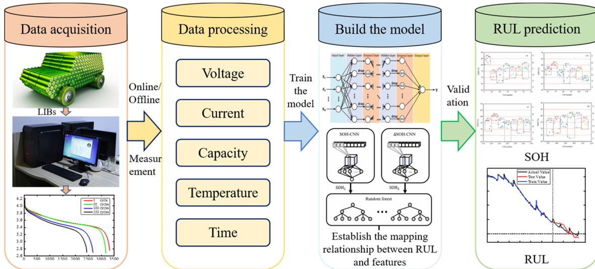
Figure 9. Framework for the data-driven approach of RUL prediction.
