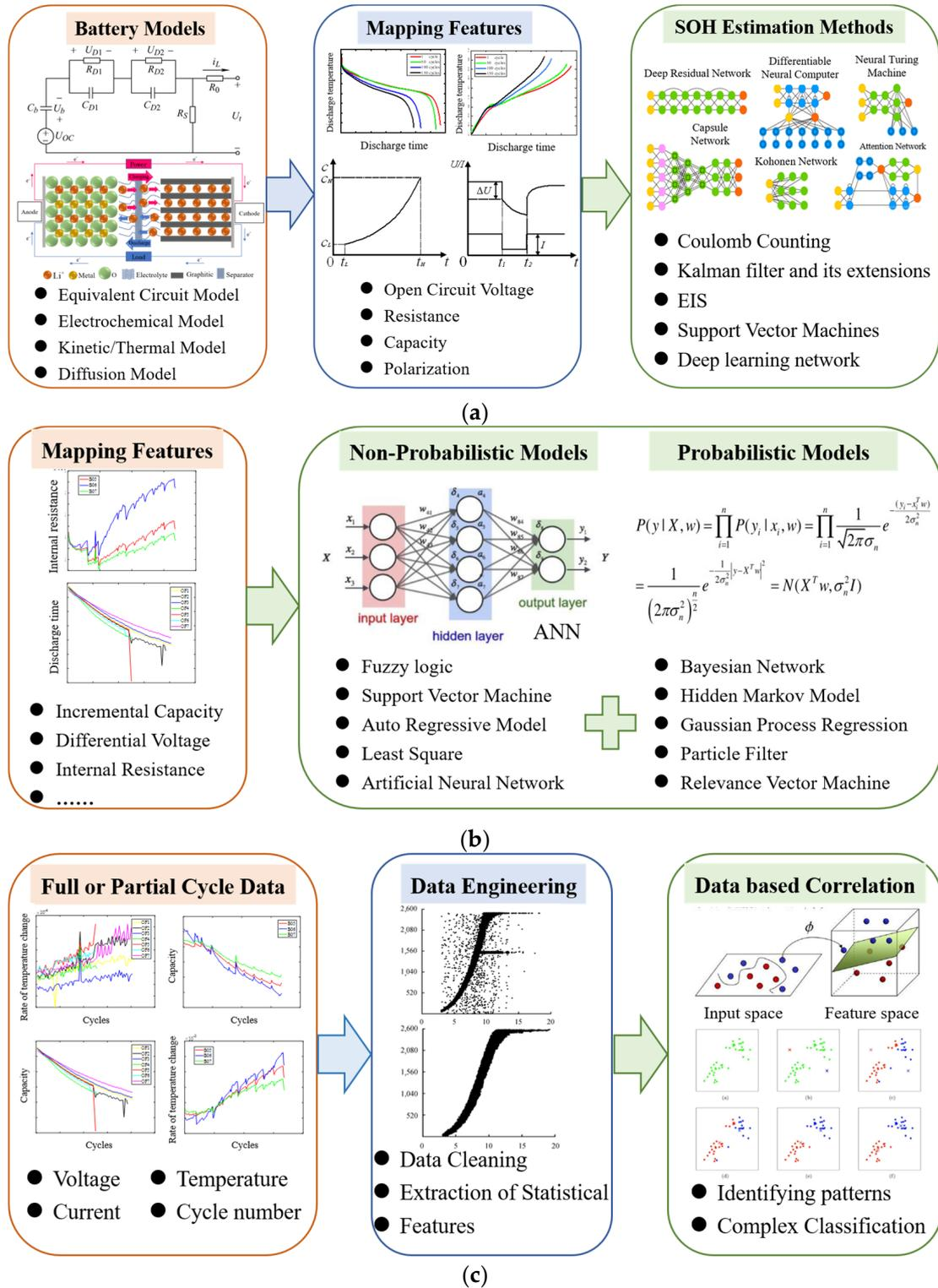
Figure 7. SOH estimation [53]. (a) Model-based features for SOH estimation. (b) Data-based analytical features for SOH estimation. (c) Battery management system-based raw features for SOH estimation.
