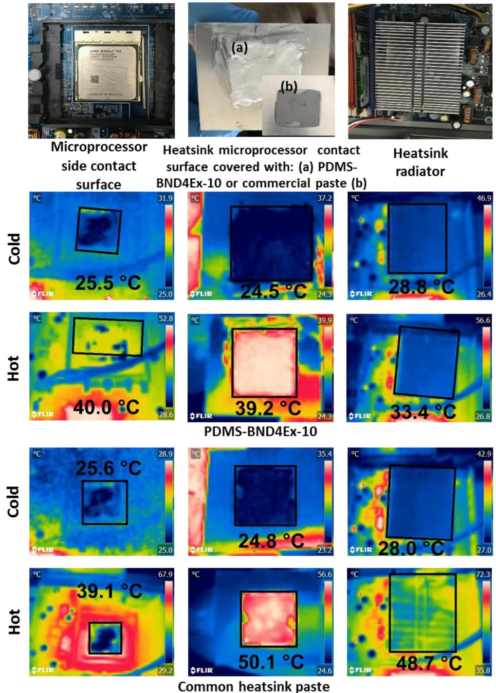
**Figure 11.** IR camera images and temperatures of the cooling surfaces tested for heat conduction of PDMS-BND4Ex-10 composite, as compared with commercial heatsink paste.
