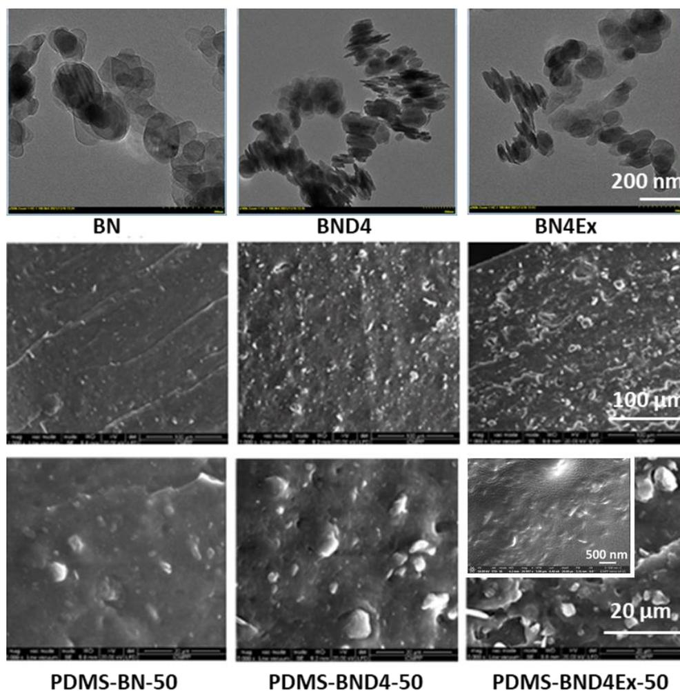
**Figure 5.** TEM images of the three varieties of BN (top) and SEM images of the derived PDMS-BN composites.
