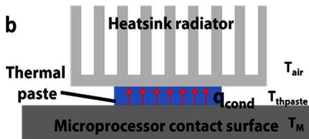
**Figure 10.** Thermogravimetric curve for the PDMS-BND4Ex-10 (top); top picture of the heatsink setup (a); schematics of the cooling setup with thermal paste (b) (down).
