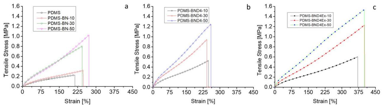
**Figure 8.** Stress–strain curves for the three composite series: (a)—with the pristine BN powder; (b)—with BN treated with D4; (c)—with BN treated with D4 and exfoliated.
