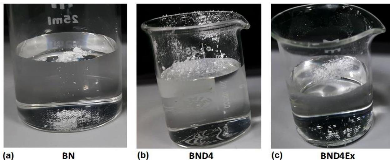
**Figure 4.** Images revealing the behavior, on contact, with water of the pristine BN powder (a) or treated differently: with D<sub>4</sub> (b) and exfoliated after hydrophobization with D<sub>4</sub> (c).
