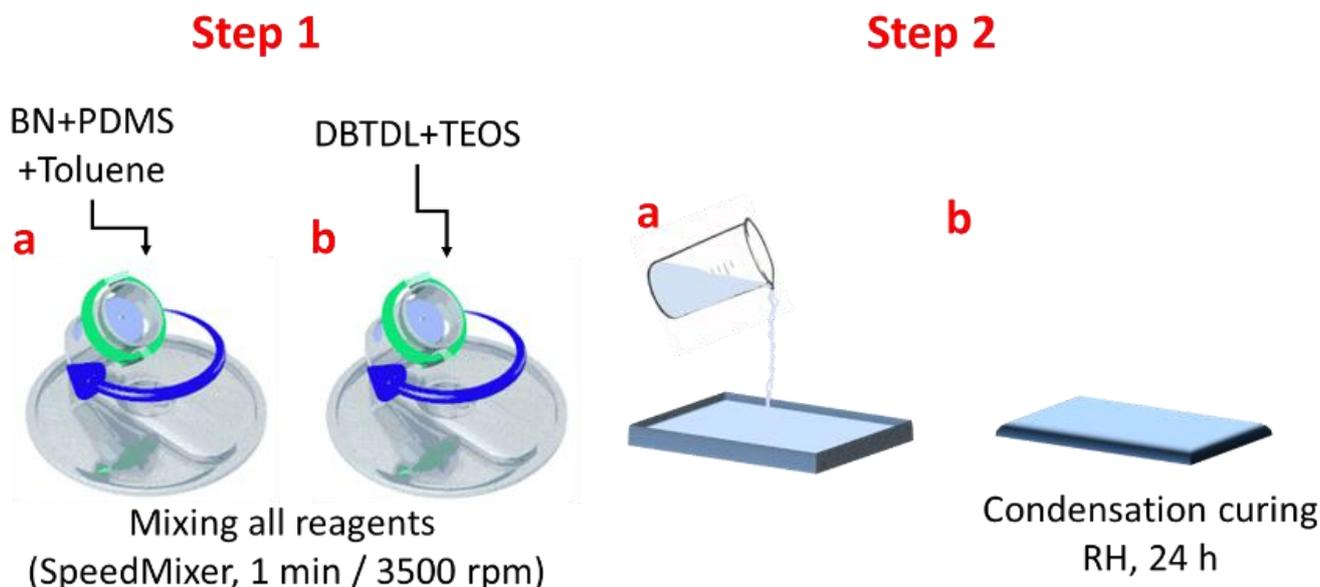
**Figure 7.** Manufacturing steps for obtaining silicone-based composites with BN.
