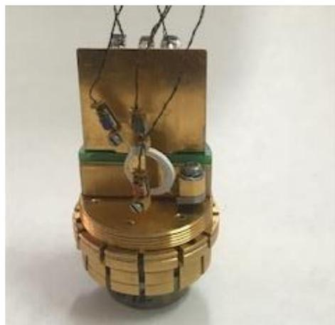
**Figure 1.** Sample assembled in the PPMS.
