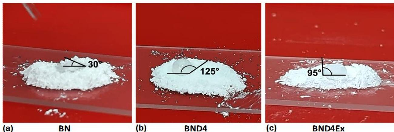
**Figure 3.** Photo images showing the shape of the water drop on the pristine BN powder (a) or treated differently: with D<sub>4</sub> (b) and exfoliated after hydrophobization with D<sub>4</sub> (c).
