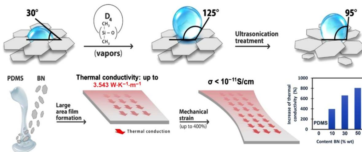
**Scheme 1.** Illustration of the protocol addressed in this work for obtaining composites for thermal management and their main performances obtained.
