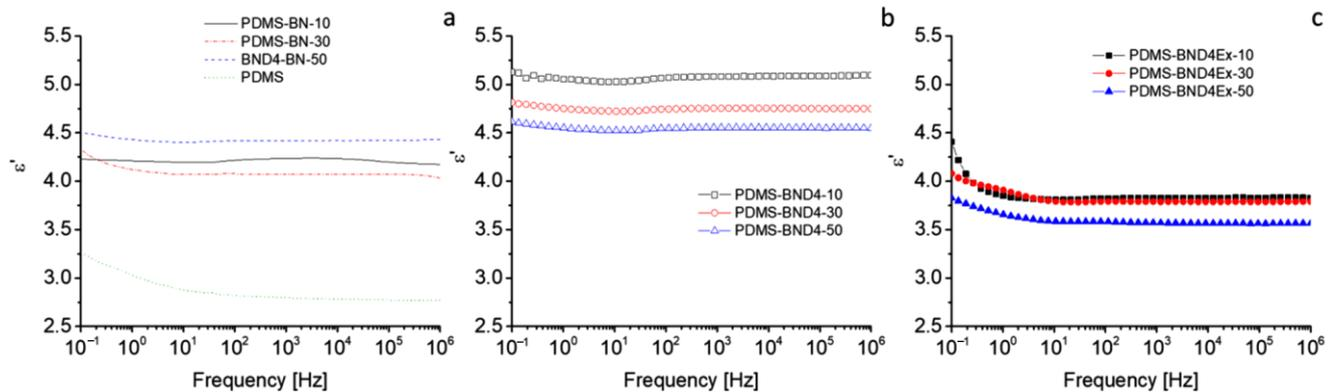
**Figure 9.** Dielectric spectra of the three composite series: (a)—with the pristine BN powder; (b)—with BN treated with D4; (c)—with BN treated with D4 and exfoliated.
