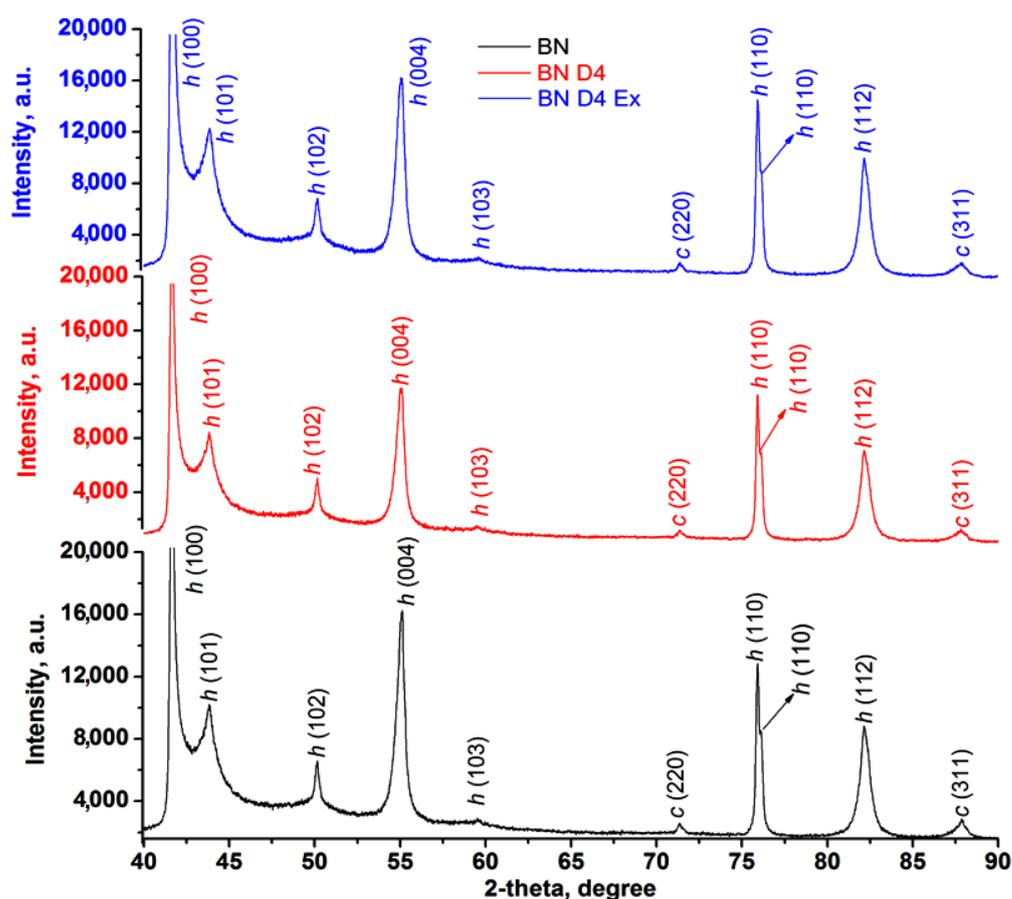
Figure 6. XRD patterns for initial, hydrophobized, and exfoliated BN particles.
