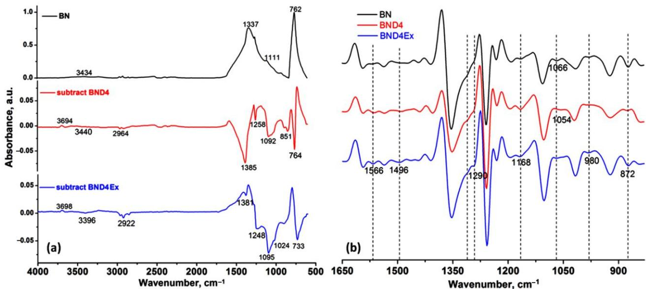
**Figure 2.** ATR-IR spectrum of BN, subtracted spectra of BND4 and BND4 Ex, (a) and the 2nd derivative of the spectra of the sample in the 1650–830  $\text{cm}^{-1}$  (b).
