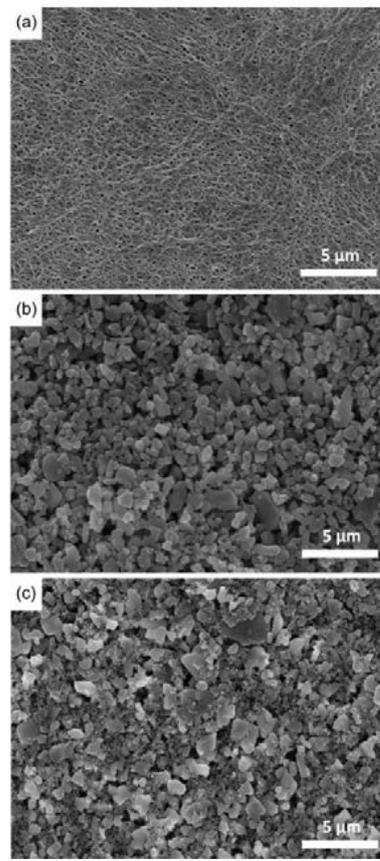
**Figure 4.** SEM images of the surfaces of (a) bare PE separators, (b) SC-CCS containing Al<sub>2</sub>O<sub>3</sub>, and (c) DC-CCSs.
