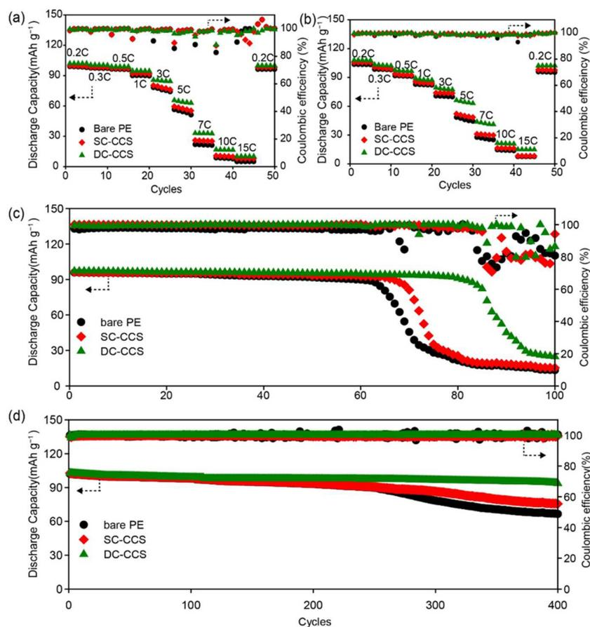
**Figure 7.** Rate capability of CR2032-type (a) half cells (LMO/Li metal) and (b) full cells (LMO/graphite) (discharging rate was varied while maintaining the charging rate of  $C/5 = 0.257 \text{ mA cm}^{-2}$ ) with the Coulombic efficiencies. Cycle performance of CR2032-type (c) half cells (LMO/Li metal) and (d) full cells (LMO/graphite) (charging and discharging rates =  $1.283 \text{ mA cm}^{-2}$ ) with the Coulombic efficiencies.
