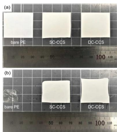
**Figure 6.** Digital camera images of bare PE, SC-CCSs, and DC-CCSs (a) before and (b) after exposure to 140 °C for 30 min.
