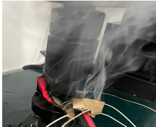
Figure 17. Side cracking of the cell during extrusion.
