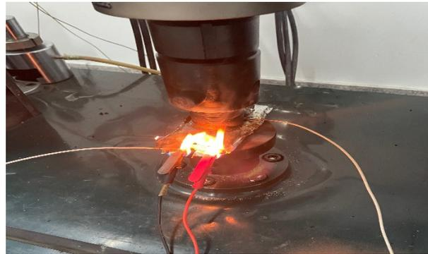
**Figure 20.** Battery fire during crash test.
