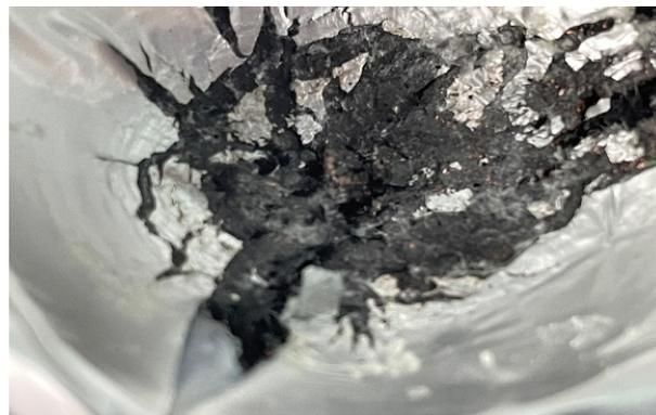
Figure 9. Internal details of the battery after the experiment.
