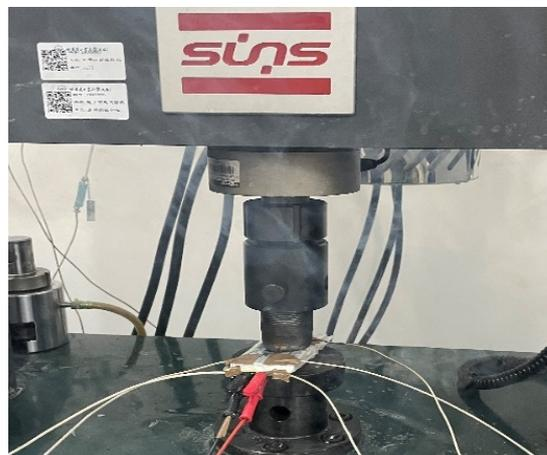
Figure 12. Smoke when the battery fails.
