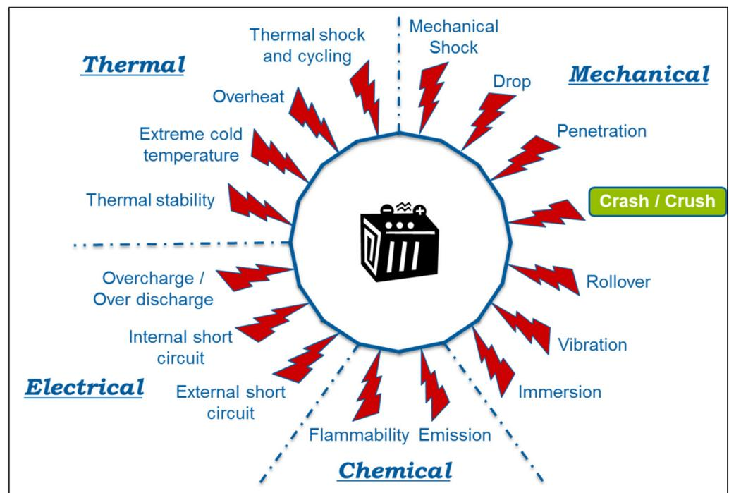
**Figure 1.** Abuse tests for the battery as per different standards and regulations [73].
