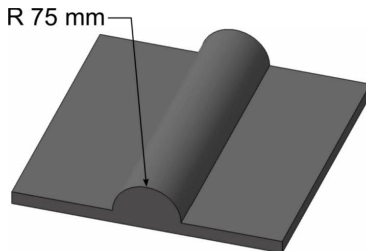
**Figure 7.** Crush plate for the module as per SAND2017-6925:2017 [107].
