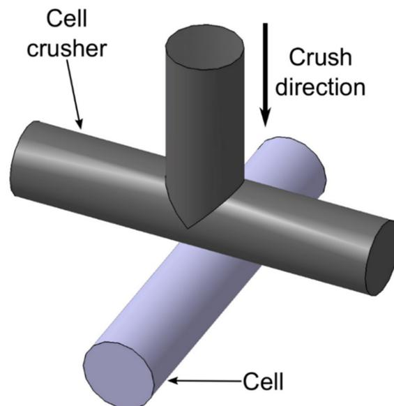
Figure 8. Cell crusher as per SAE J2464:2009 [89], FreedomCAR:2006 [92], IEC 62660-2:2010 [87], and SAND2017-6925:2017 [107].
