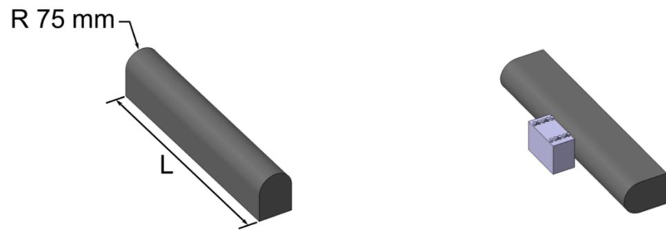
**Figure 3.** Module crush board as per GB/T 31485-2015:2015 [40].
