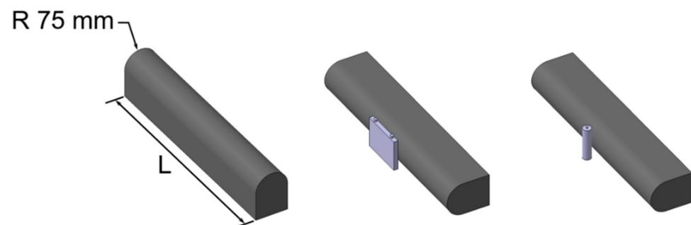
**Figure 2.** Cell crush board as per GB/T 31485-2015:2015 [40].
