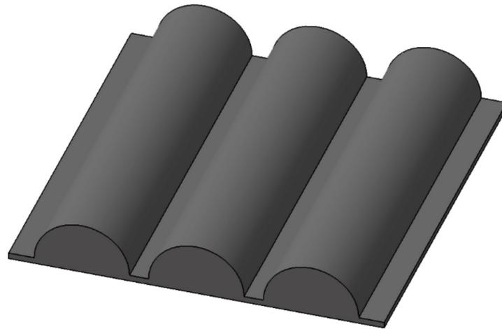
**Figure 6.** Crush plate for module as per UN/ECE-R100.02:2013 [98], GTR 20:2018 [108], SAE J2464:2009 [89], ISO 12405-3:2014 [84], and FreedomCAR:2006 [92].
