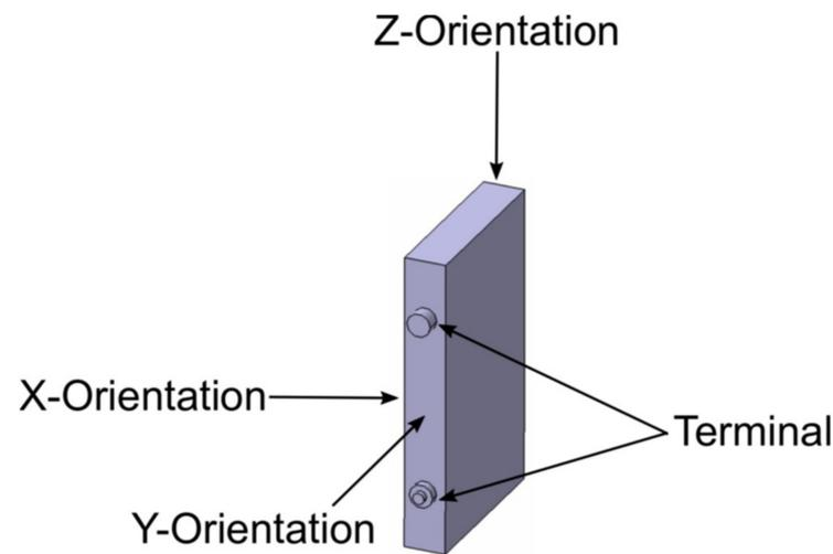
**Figure 4.** X-, Y- and Z-orientation of prismatic cell as per SAND2017-6925:2017 [107].
