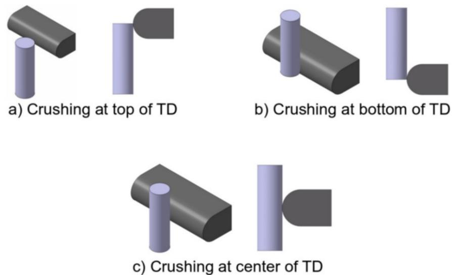
**Figure 11.** Point of contacts between impactor and TD from 3D view and front view, (a) top view; (b) bottom view; (c) centre view.
