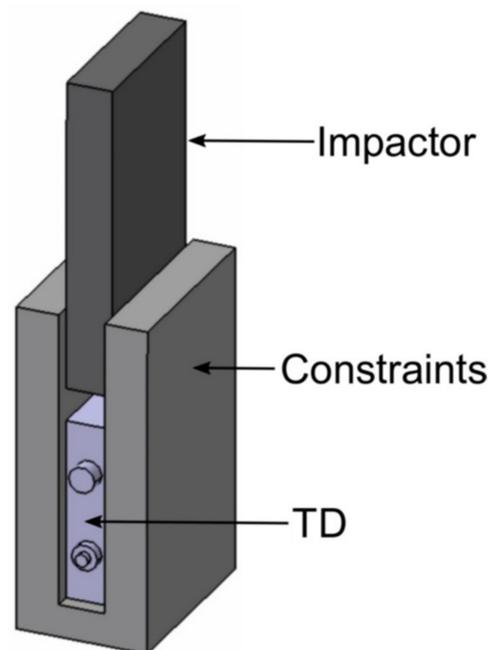
**Figure 5.** Prismatic cell in the fixture and crushed along Z-orientation as per SAND2017-6925:2017 [107].
