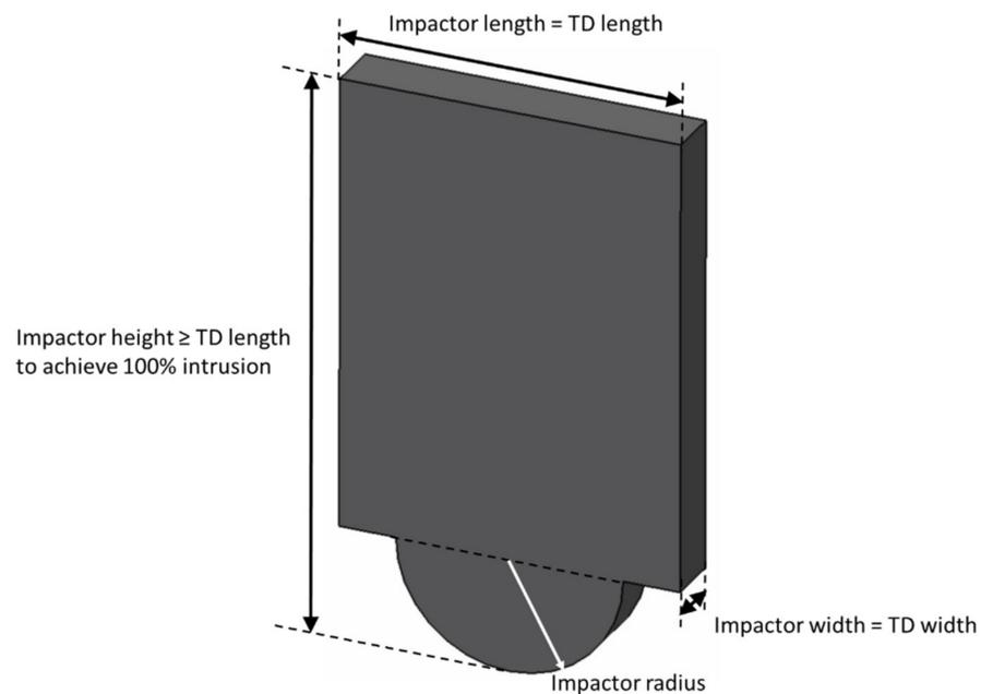
**Figure 10.** Impactor for crushing prismatic and pouch cell as per SAND2017-6925:2017 [107].**Table 7.** Recommended impactor diameter for crushing prismatic and pouch cells as per SAND2017-6925:2017 [107].
