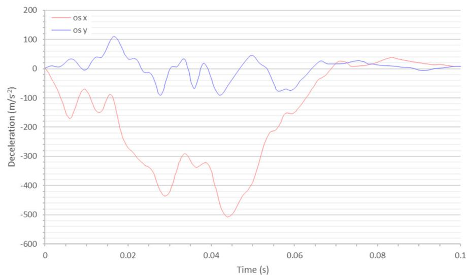
**Figure 12.** Decelerations during a crash test (speed: 54 km/h, rigid barrier, full overlap,  $0^\circ$  impact angle) [121].
