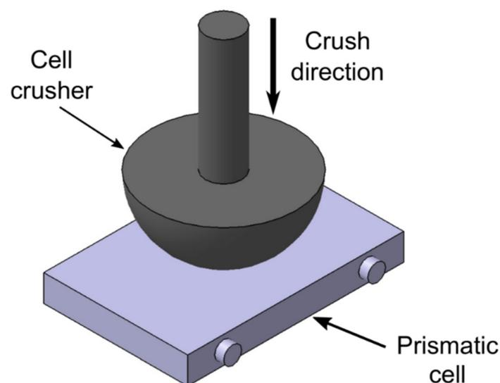
Figure 9. Cell crusher for prismatic cells as per IEC 62660-2:2010 [87].
