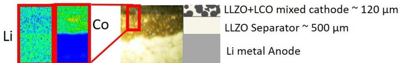
**Figure 9.** Camera image of the 4.2 V charged LLZO-based cells as seen through the beam window (**centre**) with a schematic of the cell setup (**right**) including approximate thicknesses. The red rectangle marks the analysis region of  $50 \times 300 \mu\text{m}^2$  and the resulting Co mapping by PIXE and Li mapping by PIGE (**left**).
