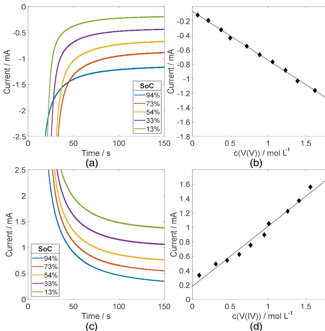
**Figure 6.** Results of chronoamperometric (CA) measurements with sensor in positive electrolyte with different SoCs; reduction current curves (a); current values versus SoC (b); oxidation current curves (c), current values versus SoC (d) ( $\pm 0.7$  V vs. open circuit voltage (OCV), platinum pseudo reference, active area  $1 \text{ cm}^2$ ).
