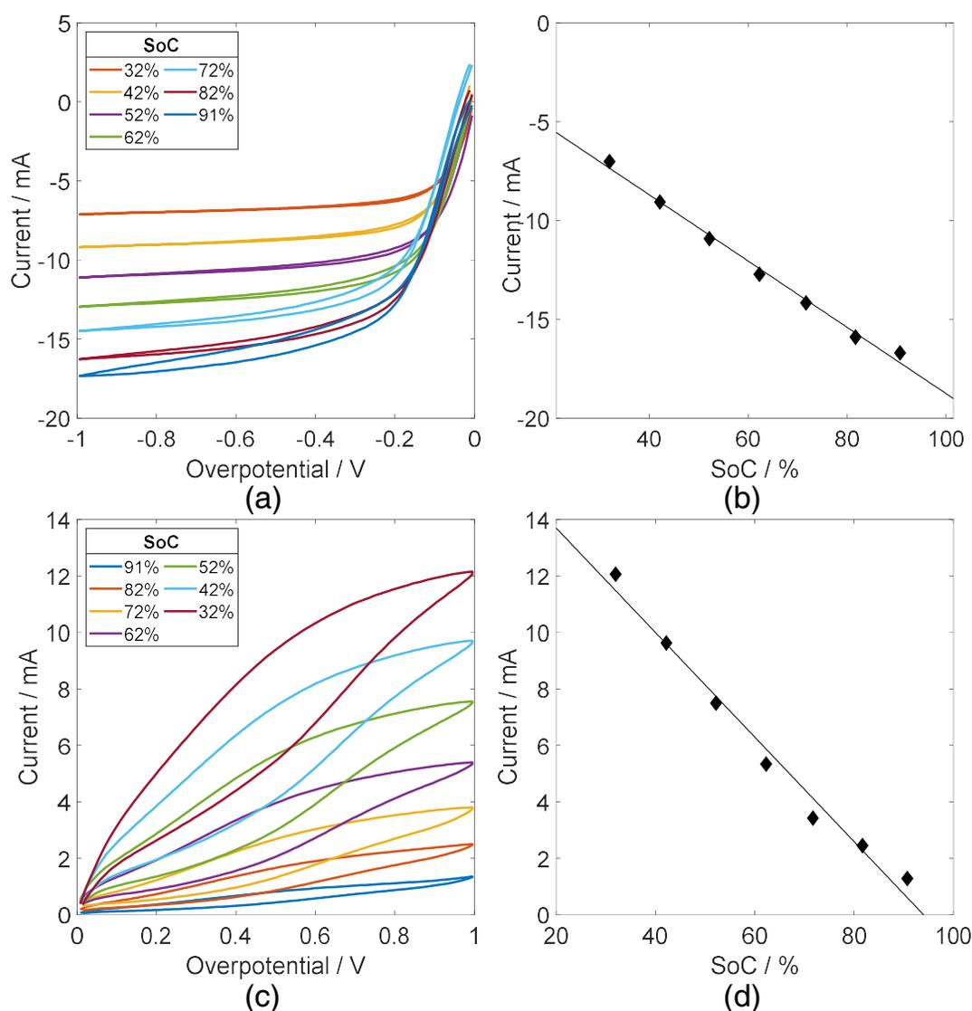
**Figure 2.** Results of cyclic voltammetry (CV) measurements with glassy carbon rotating disc electrodes (RDE) in positive electrolyte with different states of charge (SoCs), reduction current curves (a), reduction current values versus SoC (b), oxidation current curves (c), oxidation current values versus SoC (d) (scan rate 20 mV/s, platinum pseudo reference, diameter active area 5 mm).
