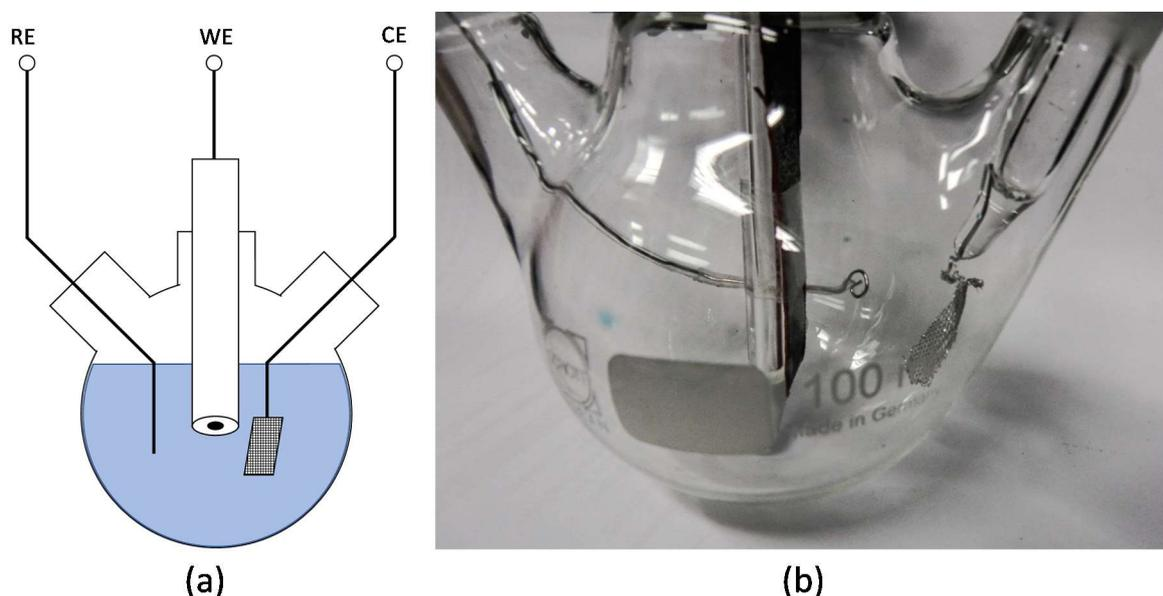
**Figure 7.** Experimental setup of rotating disc electrode (RDE) (a) and sensor (b) measurements, with RDE (diameter active area  $5 \text{ mm}$ ) or sensor (active area  $1 \text{ cm}^2$ ) as working electrode (WE), platinum mesh (approx.  $2 \text{ cm}^2$ ) as counter electrode (CE) and platinum wire as reference electrode (RE), electrolyte volume during measurement  $55 \text{ mL}$ .
