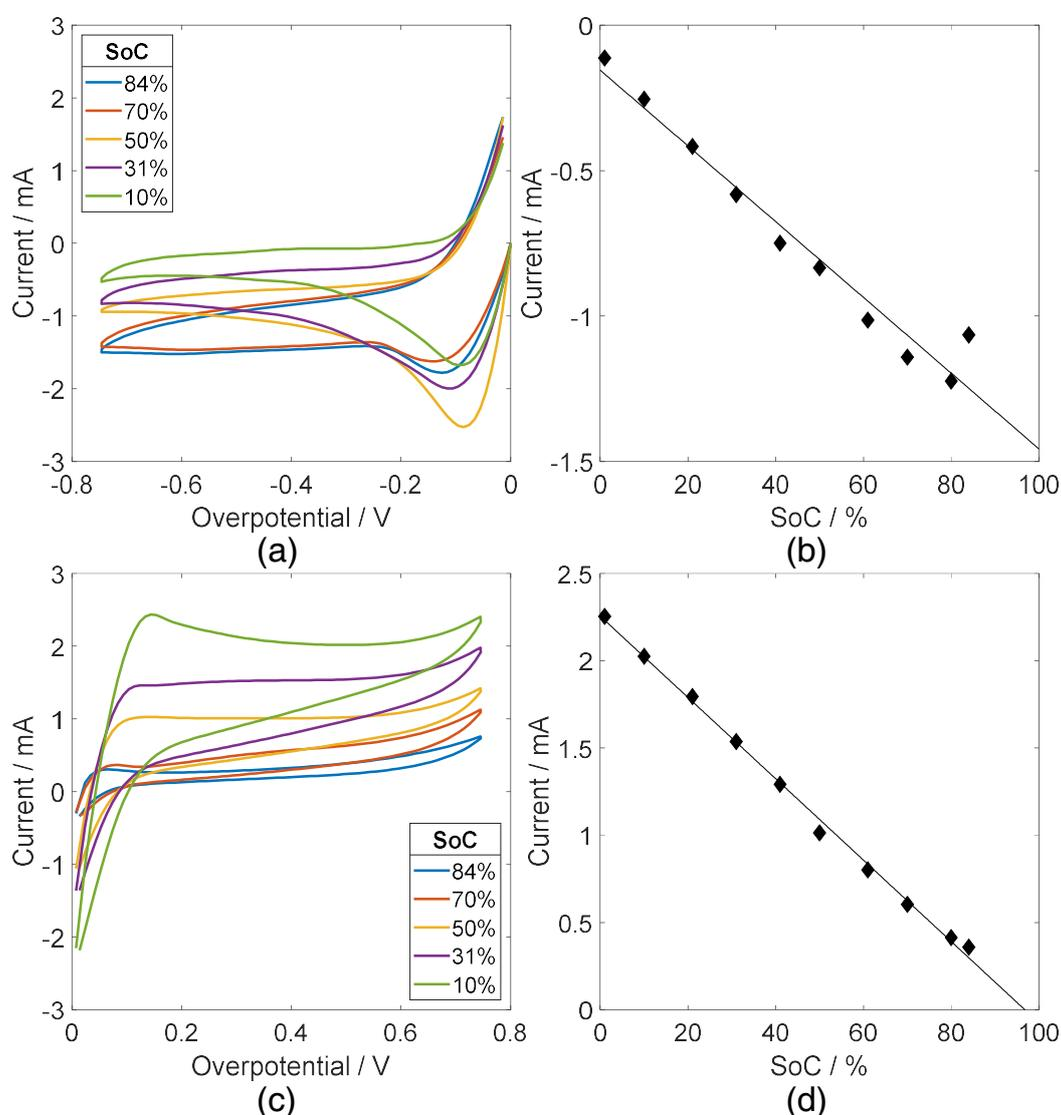
**Figure 5.** Results of CV measurements with sensor in positive electrolyte with different SoCs; reduction current curves; (a) current values versus SoC, (b) oxidation current curves, (c) current values versus SoC, (d) (scan rate 20 mV/s, platinum pseudo reference, active area 1 cm<sup>2</sup>).
