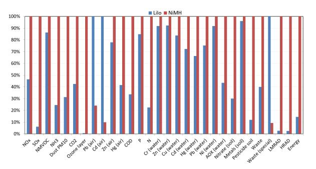
**Figure 11.** Comparison of metal and gas-based emissions of LiIo and NiMH batteries by the EcoPoints 97 method.
