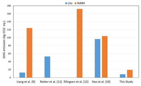
Figure 13. Comparison of the GHG emission outcomes of LiIo and NiMH batteries with existing studies.
