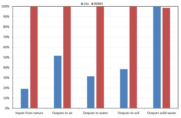
Figure 8. Comparative LCA inputs and outputs of LiIo and NiMH batteries by the RMF approach.
