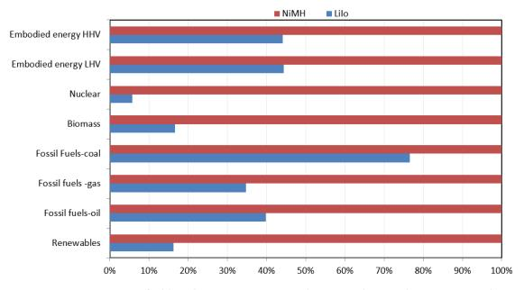
**Figure 12.** Comparative fuel-based energy consumption by LiIo and NiMH batteries, using the CED approach.
