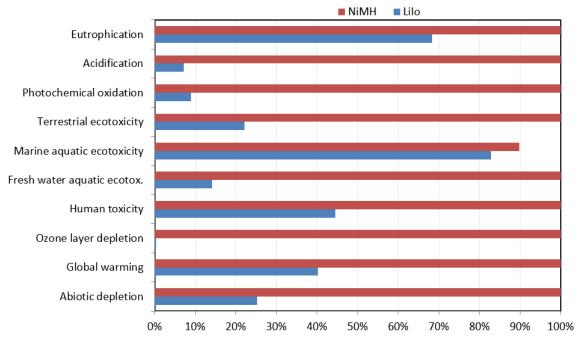
Figure 9. LCA outcome comparison per impact indicator, using the CML midpoint method.
