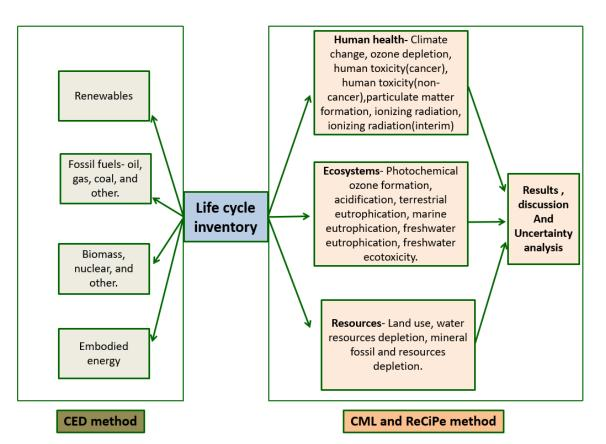
Figure 7. Schematic diagram of the CED and CML methods of LCA analysis.
