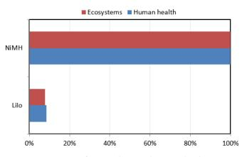
Figure 10. LCA outcome comparison of LiIo and NiMH batteries by the ReCiPe endpoint method.
