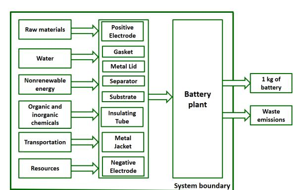
Figure 6. System boundary of the batteries for life cycle impact assessment.
