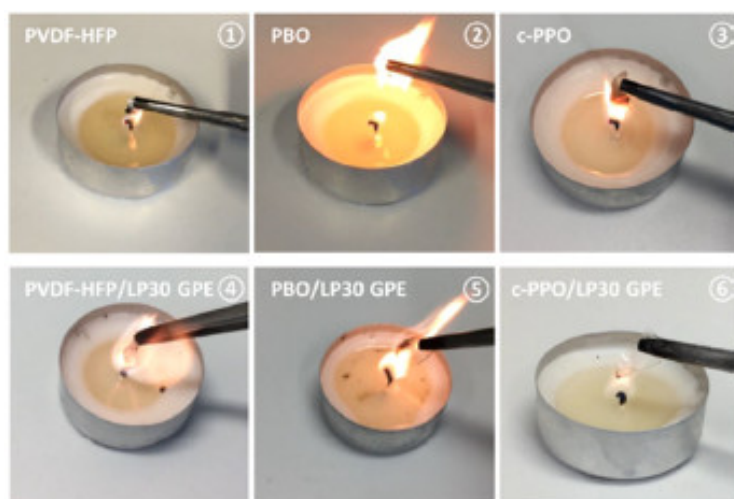
Figure 17. Flammability measurement of PVDF-HFP (polyvinylidene fluoride-hexafluoropropylene), PBO (poly [benzyl methacrylate-co-oligo(ethylene glycol) ether methacrylate]), and c-PPO (cross-linked poly[dimethyl-p-vinyl benzyl phosphonate-co-oligo (ethylene glycol) methacrylate] co-polymer) polymer matrices and their corresponding GPEs.
