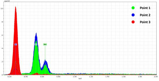
Figure S2 Energy-dispersive X-ray spectroscopy analysis
