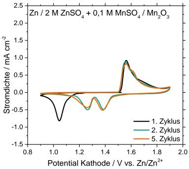
**Figure S4** CV measurements (potential sweep rate  $0.1 \text{ mV s}^{-1}$ ) of a battery with ball milled active material. The first cycle shows a sharp single reduction peak at 1.05 V and a broader oxidation peak at 1,56 V. The following cycles show two reduction (1,38 V and 1,26 V) an two oxidation peaks (1,56 V and 1,62 V) each. The broad, single oxidation peak of the first cycle seems to divide into two peaks, with one of the peaks getting formed out of the shoulder of the broad peak.
