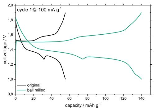
**Figure S3** Cell voltage curves showing the first cycle with an applied current density of 100 mA g<sup>-1</sup> of the cell with original (black line) and ball milled active material (green line). Two voltage plateaus each are visible in charge and discharge step (the voltage plateaus of the discharge steps are divided by a significant voltage drop), which can be dedicated to phase transformations effects.
