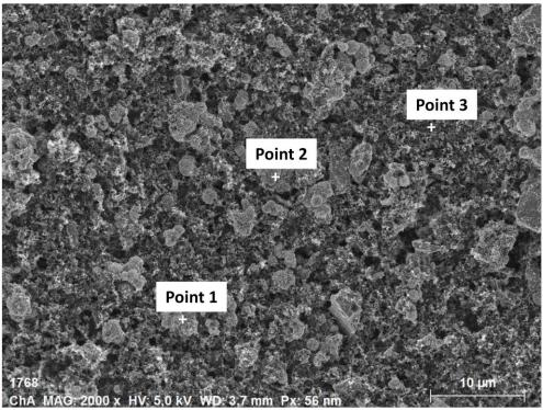
$Figure \,\,S1 \, {\rm Points} \, in \, the \, {\rm SEM} \, image \, of \, the \, cathode \, which \, were \, analyzed \, by \, {\rm Energy-dispersive} \, {\rm X-ray} \, spectroscopy$
