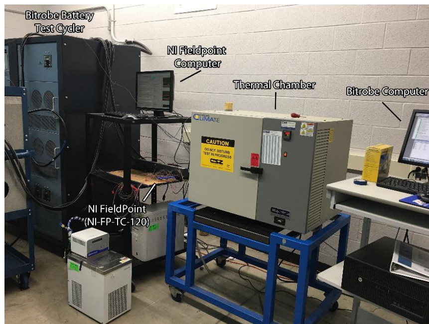
Figure 1. Experimental set-up for model development and voltage validation.
