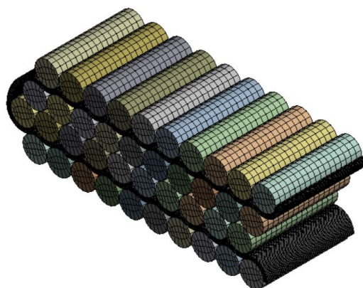
Figure 3. Mesh of the battery pack.
