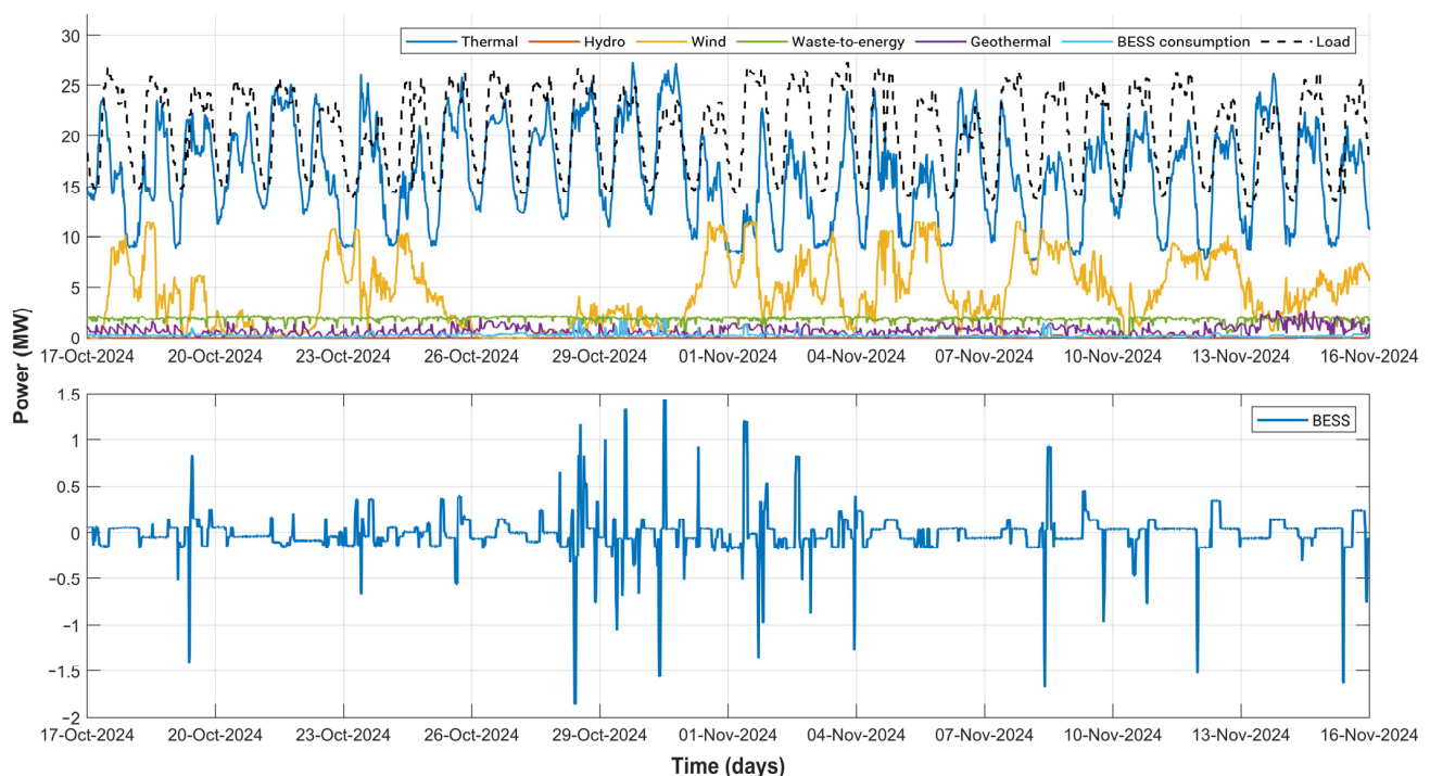
Figure 7. Power time series during 30 days of system operation (17 October–15 November 2024). Top: generation assets and system load. Bottom: net BESS power (positive and negative correspond to charging and discharging, respectively).
