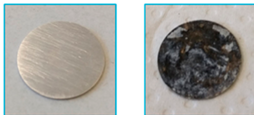
Figure 8. Pristine magnesium surface compared with surface covered by the black layer after contact with alginate solution.
