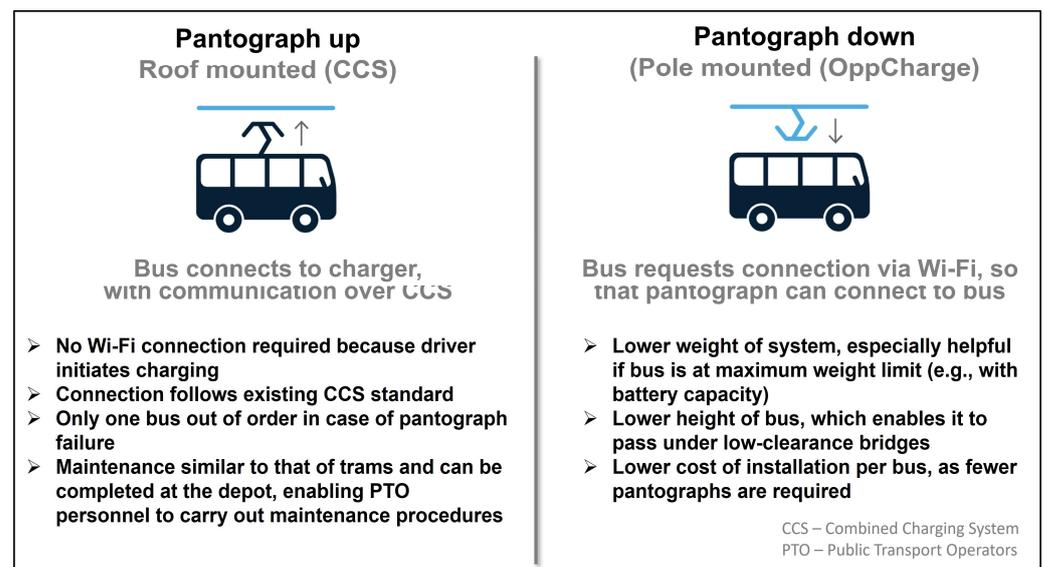
**Figure 7.** Figure illustrating the benefits of each pantograph system. Adapted from [62].
