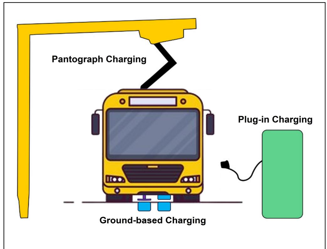
Figure 6. Illustration showing the three primary forms of charging.
