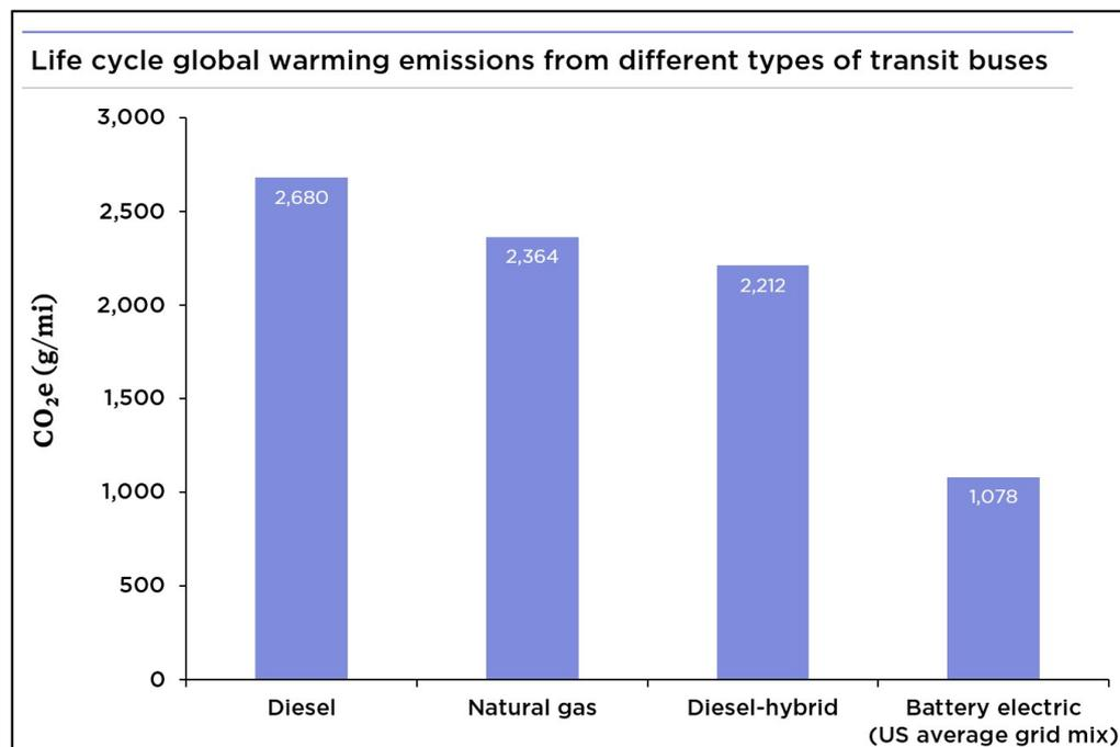
**Figure 9.** CO<sub>2</sub> emissions from buses. Reproduced with permission from [81].
