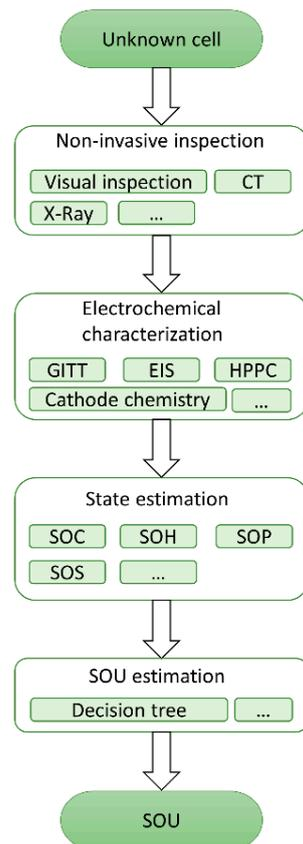
**Figure 4.** Flow chart of the SOU determination procedure. Each block may contain additional or different experimental and estimation techniques.
