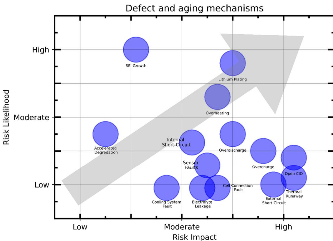
**Figure 1.** Assessment of possible risk for relevant defect and aging mechanisms in lithium-ion batteries.
