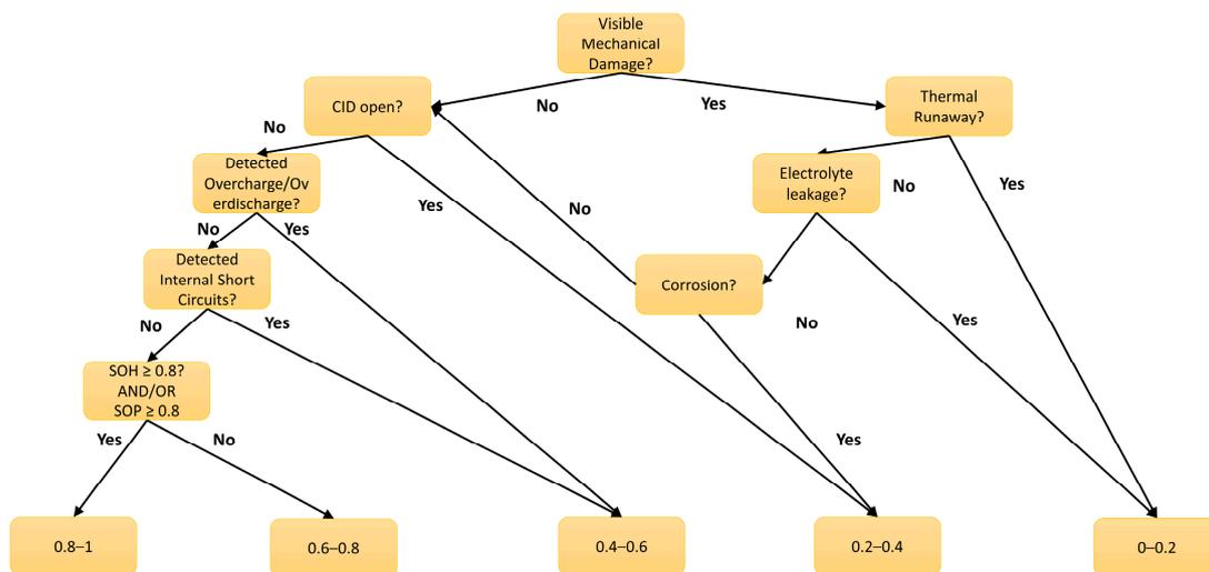
**Figure 2.** Decision tree for quick characterization of usability of used battery cells or packs.
