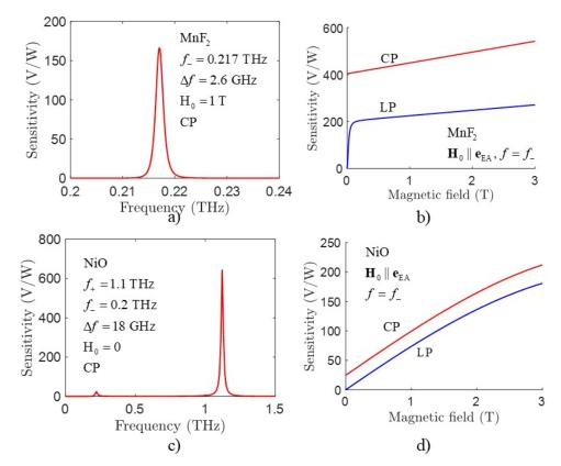
**Figure 2.** AFM detector sensitivity as a function of the external signal frequency  $(\mathbf{a}, \mathbf{c})$  and bias magnetic field  $(\mathbf{b}, \mathbf{d})$  for the AFM-HM heterstructures containing uniaxial  $(MnF_2)$  and biaxial (NiO) AFM crystals. Calculation were performed for the lowest-frequency AFMR modes).
