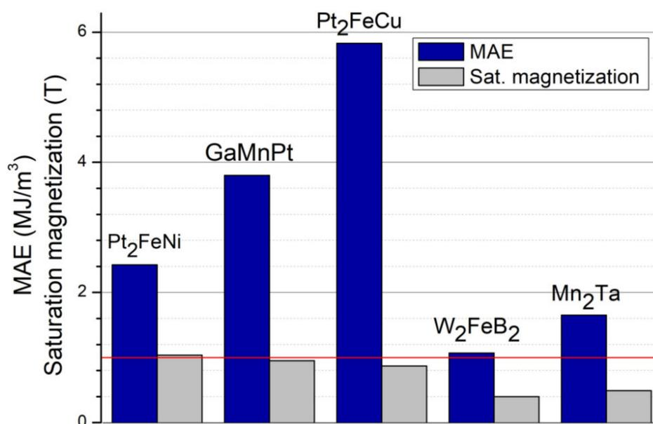
**Figure 2.** Magnetocrystalline anisotropy energy and saturation magnetization (polarization) of previously researched (Pt<sub>2</sub>FeNi) of potential candidates for PM. Red line indicates the threshold for a potentially successful PM. Further information available in [16]. This article or its components is available under the terms of the Creative Commons Attribution 4.0 International License (<https://creativecommons.org/licenses/by-nc-sa/4.0/> accessed on 12 March 2021).
