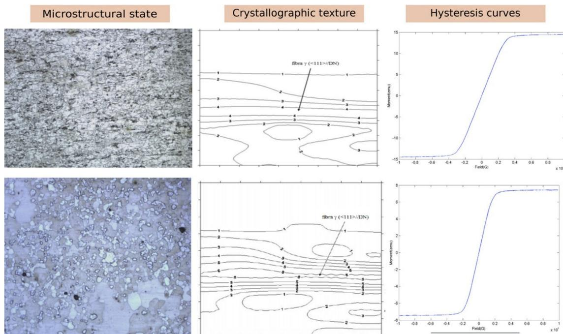
**Figure 8.** Conventional forms of characterization typically implemented in the manufacturing of electrical steels. Micrographs have been used to separate lower- and higher-efficiency materials [24]. This article is published under the terms of the Creative Commons Attribution-Non-Commercial-No Derivatives License (CC BY NC ND) (<https://creativecommons.org/licenses/by-nc-nd/4.0/> accessed on 12 March 2021).
