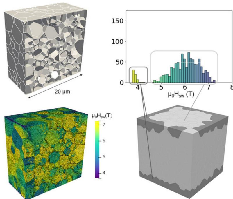
**Figure 5.** Representation of structure with identification of grain with lower switching fields (positioned on the edges) [21]. This article is licensed under a Creative Commons Attribution 3.0 License (<https://creativecommons.org/licenses/by/3.0/> accessed on 12 March 2021).
