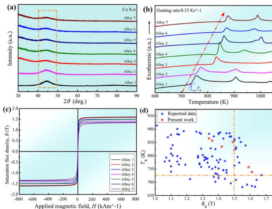
**Figure 4.** (a) X-ray diffraction patterns, (b) differential scanning calorimetry curves, (c) hysteresis loops, and (d) saturation polarization and  $T_x$  of designed (modeled via ML) and experimental Fe-based metallic glasses. Further information available in [20]. This article is licensed under a Creative Commons Attribution 4.0 International License (<https://creativecommons.org/licenses/by-nc-sa/4.0/> accessed on 12 March 2021).
