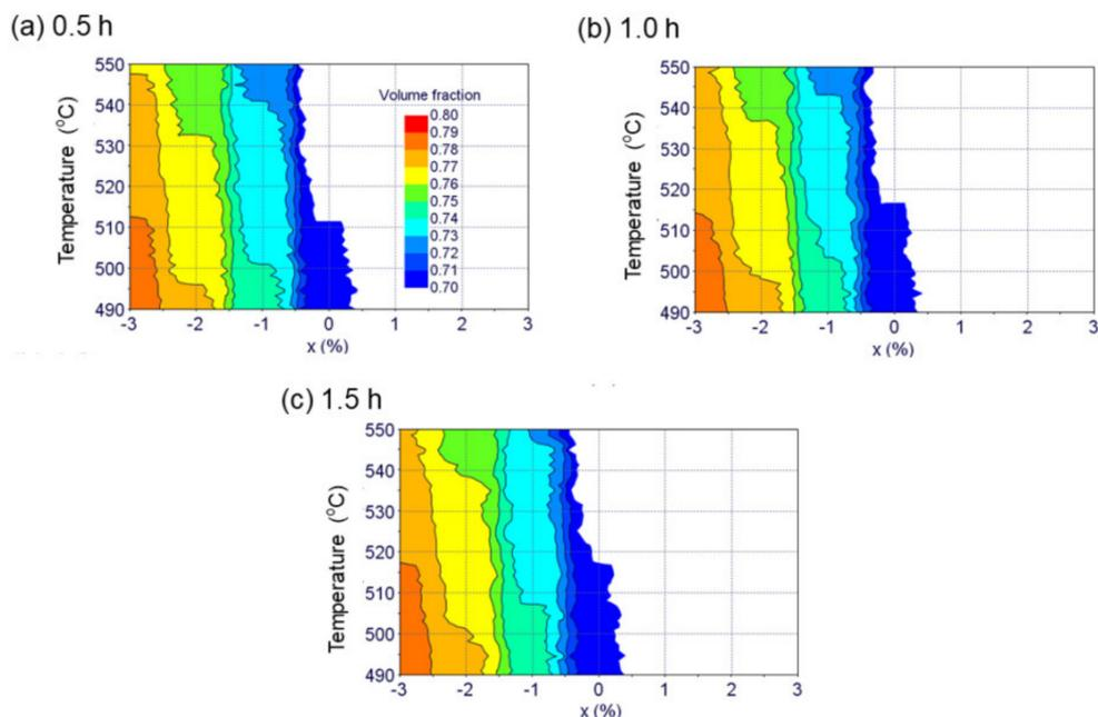
**Figure 7.** Example of volume fractions of nanocrystalline phase predicted after distinct periods of annealing time ((a): 0.5 h; (b): 1.0 h; (c): 1.5 h) as a function of different Fe and Si (x %) content [23]. Reprinted with permission from Elsevier.
