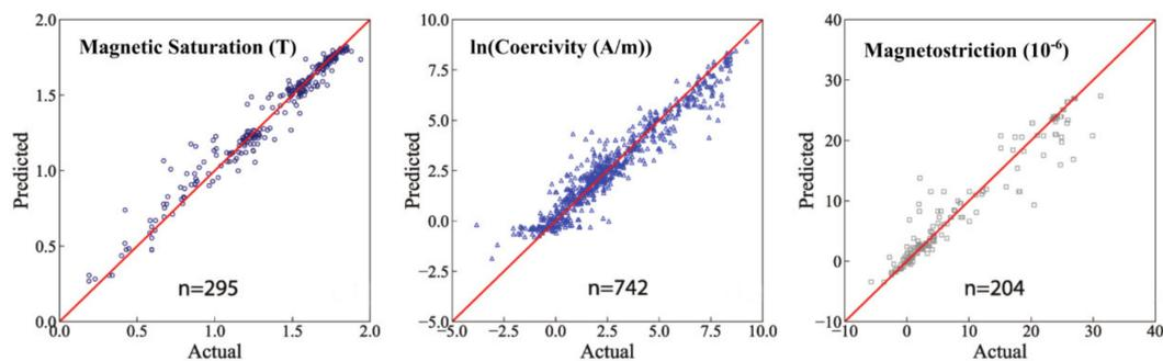
**Figure 3.** Experimental versus predicted (via machine learning) values of magnetic saturation (polarization), coercivity, and magnetostriction for Finemet-type soft magnetic alloys. Further information available in [19]. Reprinted with permission from Elsevier.
