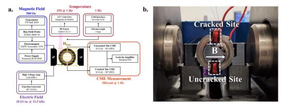
**Figure 3.** (a) Schematic diagram overview of the experimental setup including loading and sampling parameters, and (b) multiferroic composite cylinder in the testing configuration with electromagnet poles, a coil mount, and CME coils visible.
