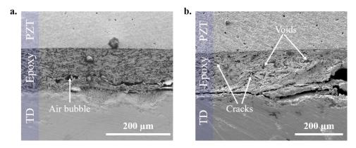
**Figure 6.** SEM micrograph of the epoxy interface sandwiched between the magnetostrictive Terfenol-D and piezoelectric PZT layers (**a**) before electrically and magnetically loading the sample and (**b**) after the 45-day period of cyclic loading.
