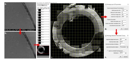
**Figure 2.** SEM image reconstruction process using ImageJ2/TrakEM2, where (**a**) an original SEM micrograph was (**b**) cropped with removed labels, (**c**) the approximate alignment of the image was set using a square grid, (**d**) SIFT parameters were used for feature detection, and (**e**) geometric consensus filter parameters were used to control the tile alignment.
