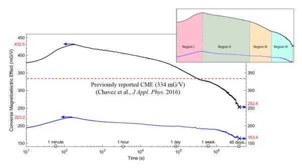
**Figure 7.** CME response for cracked (blue) and uncracked (black) sites and the previously reported CME of identical cylinder structure under short-term loading ([12]) is shown as a red dashed line. A time lag was observed between the initial response peaks of cracked and uncracked sites. The inset shows the regions of the magnetoelectric response.
