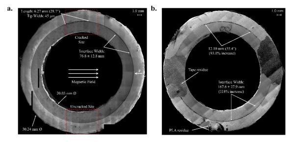
**Figure 4.** Stitched SEM images of the multiferroic cylinder composite (**a**) before testing, where the region of the predefined crack is annotated (here, black squares are areas of missing image data), and (**b**) after the 45-day period of cyclic loading. Degradation of the epoxy interface quality is clearly visible, as evidenced by the widespread void formation and initial crack lengthening.
