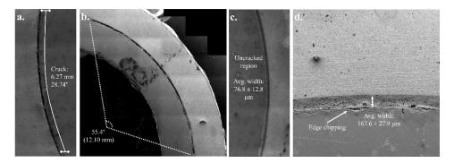
**Figure 5.** A collection of SEM micrographs of selected areas before and after the testing showing (a) the arc length of the predefined crack before testing of 6.27 mm, which (b) extended to 12.10 mm after 45 days of continuous loading, (c) a close-up view of the bonding layer showing the initial thickness of 76.8  $\pm$  12.8  $\mu$ m, and (d) the thickness of the bonding layer that had increased to 167.6  $\pm$  27.9  $\mu$ m after the testing.
