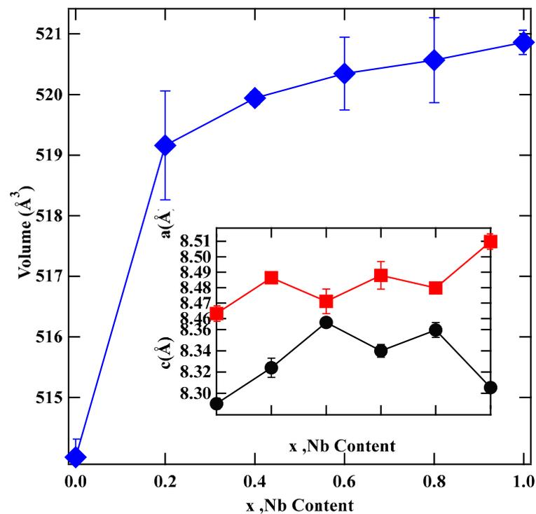
**Figure 2.** Lattice parameter  $a$  and  $c$  with the unit cell volume of  $\text{Dy}_2\text{Fe}_{16}\text{Ga}_{1-x}\text{Nb}_x$  as a function of  $x$ , Nb content.
