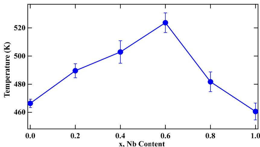
Figure 5. Curie temperature as a function of  $x$ , Nb content.
