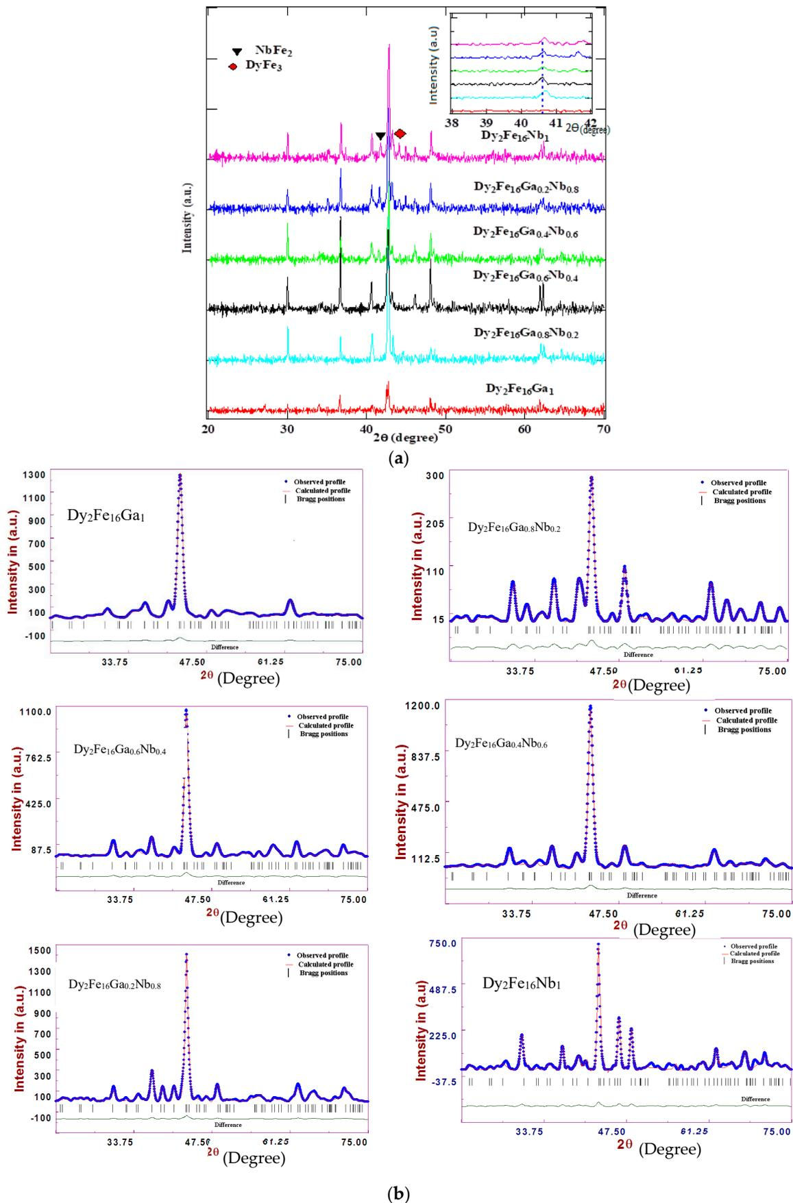
**Figure 1.** (a) X-ray diffraction patterns of  $\text{Dy}_2\text{Fe}_{16}\text{Ga}_{1-x}\text{Nb}_x$  compounds. (b) Rietveld refinement profile for  $\text{Dy}_2\text{Fe}_{16}\text{Ga}_{1-x}\text{Nb}_x$ .
