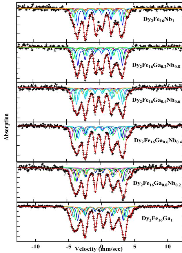
Figure 6. RT Mössbauer fitted spectra for  $\text{Dy}_2\text{Fe}_{16}\text{Ga}_{1-x}\text{Nb}_x$ .
