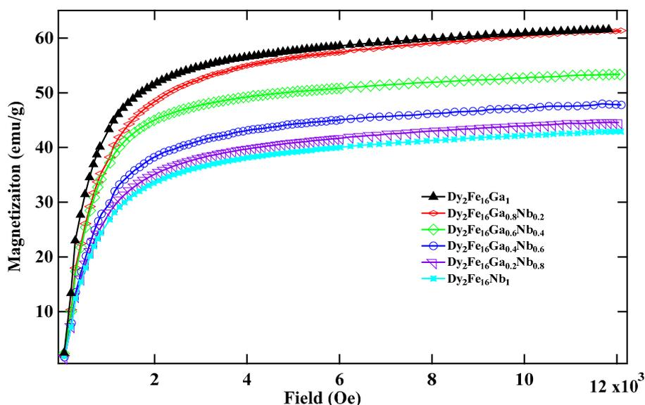
Figure 3. RT magnetization plot for  $\text{Dy}_2\text{Fe}_{16}\text{Ga}_{1-x}\text{Nb}_x$ .
