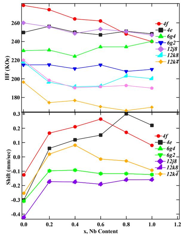
Figure 7. RT Mössbauer hyperfine parameters and isomer shift plots as a function of  $x$ , Nb content.
