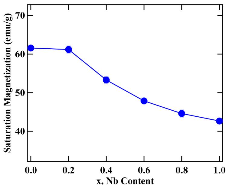
Figure 4. Room temperature (RT) saturation magnetization,  $M_s$ , as a function of  $x$ , Nb content.
