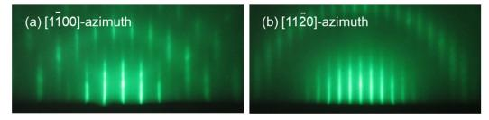
Figure 1. Reflection high-energy electron diffraction RHEED images of  $Cr_2O_3$  layer with (a)  $[1\bar{1}00]$  and (b)  $[11\bar{2}0]$  azimuth.
