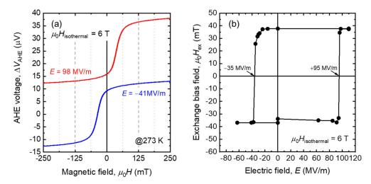
**Figure 5.** (a) AHE loops as a function of  $\mu_0 H$  after the applying the magnetoelectric (ME) fields in an isothermal way. Blue and red curves represent the AHE loop after applying E = +98 MV/m and -41 MV/m with  $\mu_0 H_{\text{isothermal}} = 6 \text{ T}$ , respectively. (b) Change in the exchange bias field as a function of E with  $\mu_0 H_{\text{isothermal}} = 6 \text{ T}$ . In (b), the threshold electric field is shown by text.
