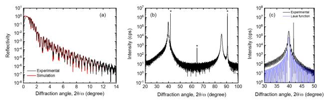
**Figure 2.** (a) X-ray reflection (XRR), (b) high-angle  $2\theta/\omega$  profile of the film. (c) represents the enlarged profile of (b) around  $2\theta/\omega = 30-50^\circ$ . Black and red lines in (a) represent the experimental result and the fitted result, respectively. Blue line in (c) represent the calculated profile using the Laue function.
