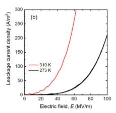
**Figure 3.** (a) Optical microscope image of the device used for the test and the electric circuitry. (b) I-V curves of the  $Cr_2O_3$  layer measured at 310 K (red) and 273 K (black).
