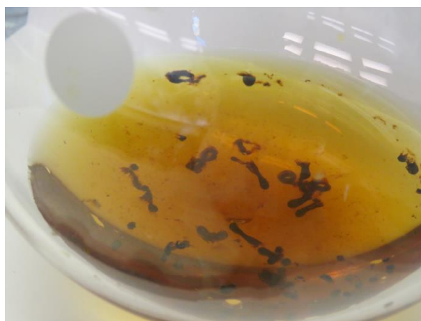
Figure 5. Iron oxide clumps observed during synthesis using conventional chemical coprecipitation with the addition of 0.4 M \text{NaOH}(\text{aq}) to an iron salt solution (90 mM \Sigma\text{Fe} ).
