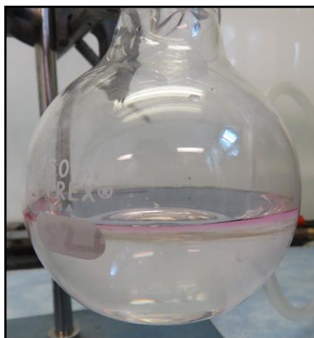
Figure 2. \text{NH}_3(\text{g}) (3.3% v/v ) headspace and aqueous solution with phenolphthalein indicator dye (0.001%) after 2 min. Phenolphthalein indicator dye is colorless <\text{pH } 8.2 and pink/red >\text{pH } 8.2 .
