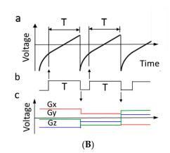
**Figure 1.** (**A**) Schematic of the in vivo digital EPR imager [26]; (**B**) timing chart and signals for the (**a**) field scan, (**b**) trigger pulse used for the data acquisition window with a period of T, and (**c**) 3D field gradients Gx, Gy, and Gz.
