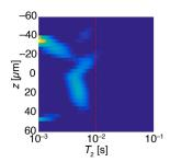
**Figure 2.** A z- $T_2$  map of a thick ( $\sim$ 100  $\mu$ m) coating sample containing 1% triphenylphosphine (PPh<sub>3</sub>). The top surface, exposed to the most intense UV irradiation, is more completely cured and shows greater crosslinking (smaller  $T_2$  values). UV does not penetrate well into the lower regions of the sample (towards the positive z direction), as indicated by the larger  $T_2$  relaxation times.
