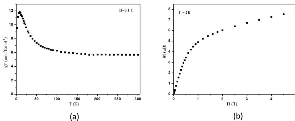
**Figure 2.** Magnetic behavior of a polycrystalline sample. (a) Temperature dependence of the product of the magnetic susceptibility with temperature ( $\chi T$ ) under an applied field of 0.1 T. (b) Field dependence of magnetization at 2 K.
