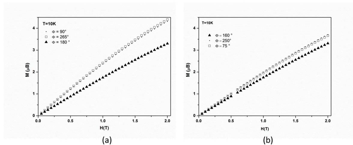
**Figure 5.** Dependence of the magnetization at 10 K with the magnetic field at the maxima and minima of the  $\chi T(\Phi)$  curves: **a**) for the rotation around the  $\vec{c}$  axis and **b**) for the rotation around the  $\vec{b}$  axis.
