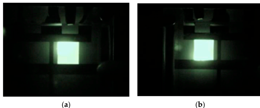
Figure 2. Photographs of the electroluminescence of (a) device I and (b) device II at 1.0 V. The cut-off wavelength is 700 nm.
