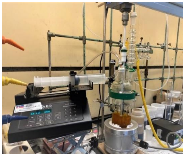
Figure S2. Experimental apparatus for the synthesis of Lignin@Fe 3 O 4 nanoparticles.
