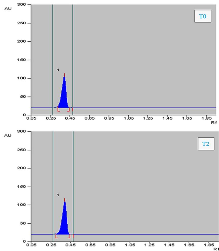
Figure 5. HPTLC densitograms of lycorine in leaf extracts in control T0 and T2 treatment of MJ.
