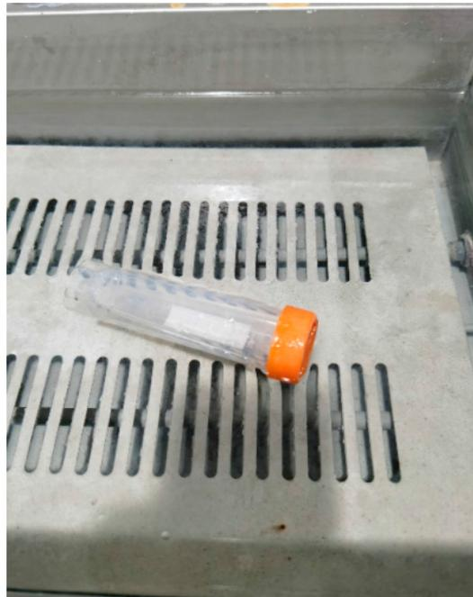
**Figure 2.** Place the centrifuge tube containing the pollen suspension into the water bath. Once positioned, secure the water bath by closing its lid.
