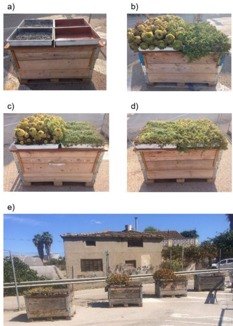
**Figure 2.** Experimental roofs over structures composed of two attached cabins covered with: (a) conventional covers: coarse gravel and red-polymer; green covers: (b) *Aeonium* and *Aptenia*, (c) *Aeonium* and *Sedum*, (d) *Sedum* and *Aptenia*; (e) general view of the distribution of four structures of the eight of the experiment.
