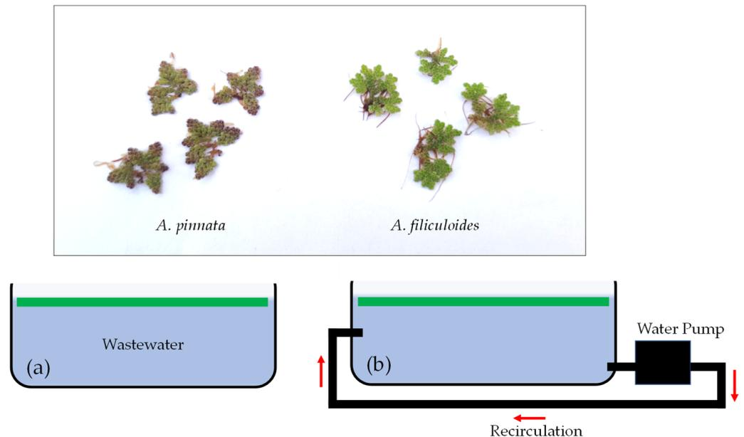
**Figure 2.** Experimental layout of (a) stagnant and (b) flowing tank reactors for the treatment of MFW using two *Azolla* spp. (Photographs: Pankaj Kumar and Ashish Kumar Arya).
