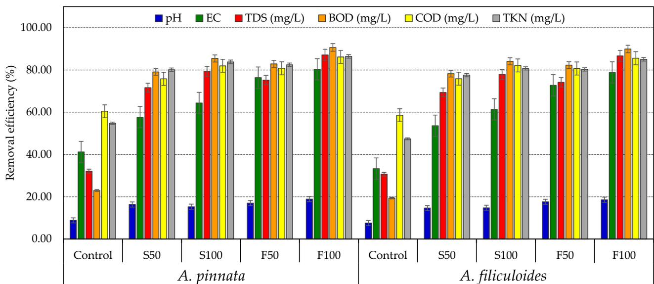
**Figure 3.** Pollutant removal efficiency of two *Azolla* spp. cultivated in different treatments of MFW (S: stagnant; F: flowing reactor).
