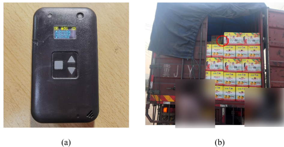
Figure 4. Truck acceleration collection test: (a) Accelerometer. (b) The position of the accelerometer in the truck.
