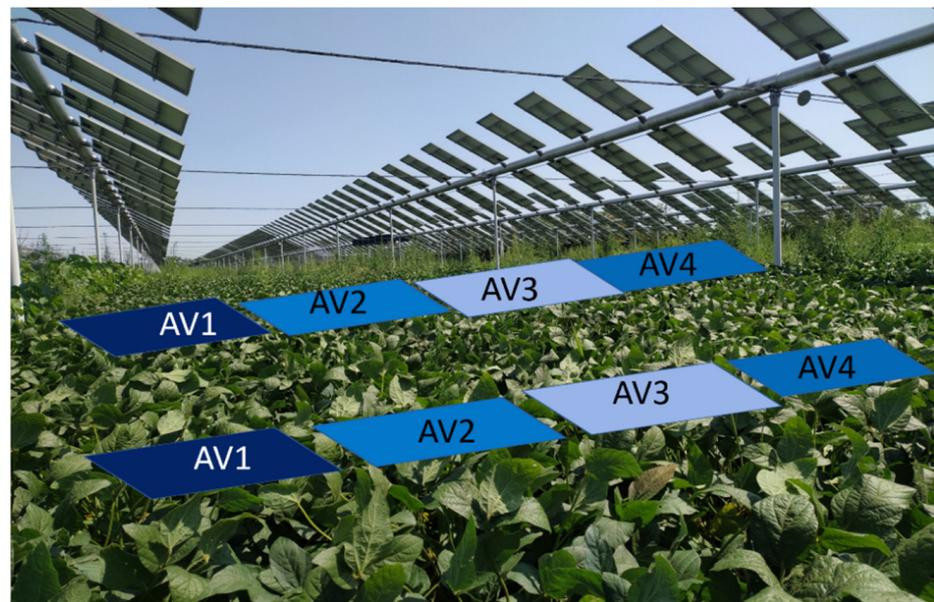
**Figure 1.** Experimental setup of the soybean trial in Monticelli D'Ongina (2021). Different colours represent the different shade depth (SD) levels, and the four SD levels are indicated as follows: AV1 = 27%, AV2 = 16%, AV3 = 9%, and AV4 = 18%.
