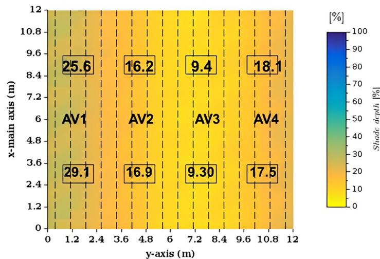
**Figure 3.** Mapped values of radiation reduction “Shade Depth (%)”. The vertical dotted lines represent crop rows, and the boxes represent the positioning and size of the plots.
