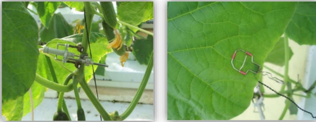
Figure 4. Stem micro-variation sensor (left) and a contact leaf temperature sensor (right).
